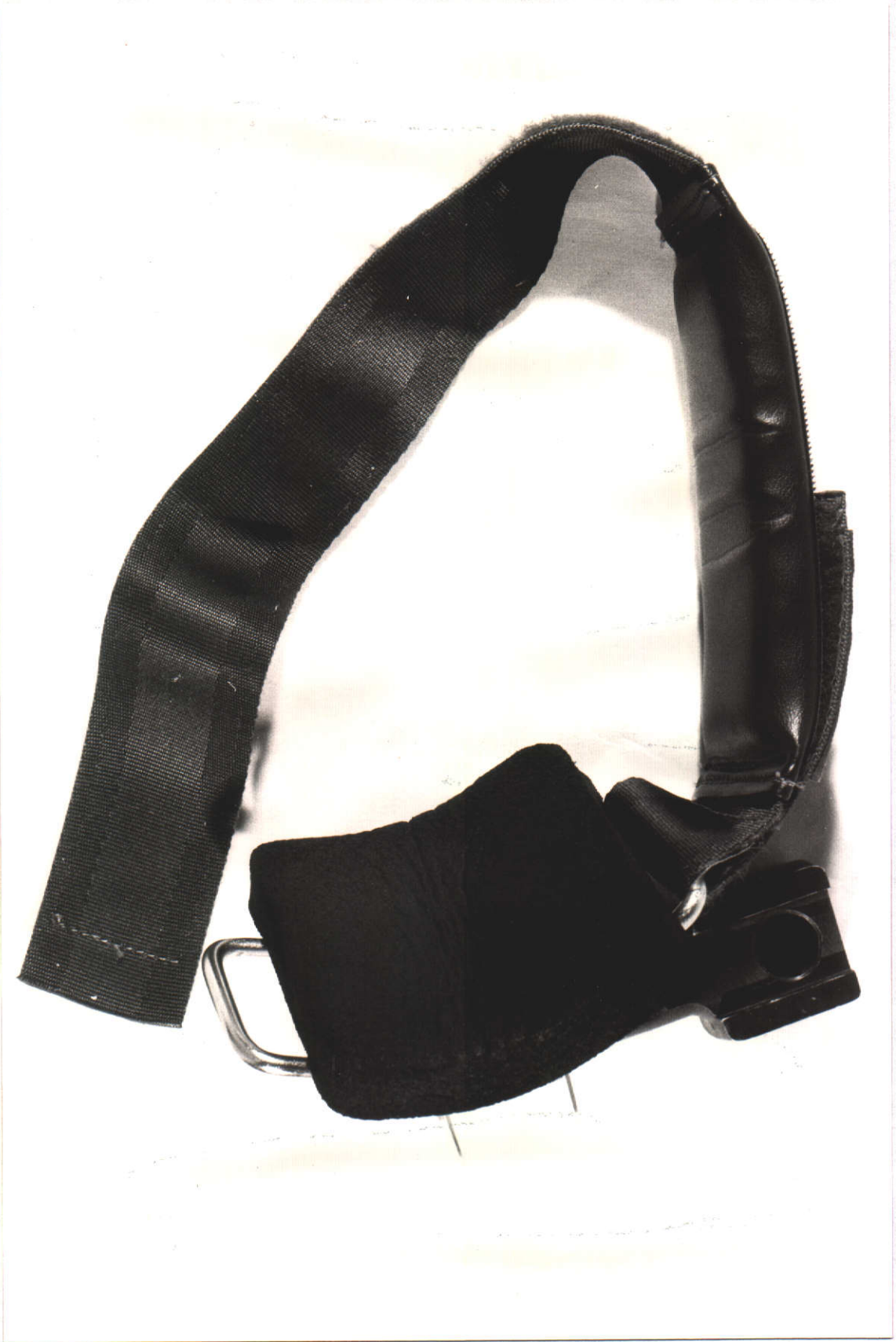
Figure 2.6 Upper extremity cuff used in isokinetic strength testing.
