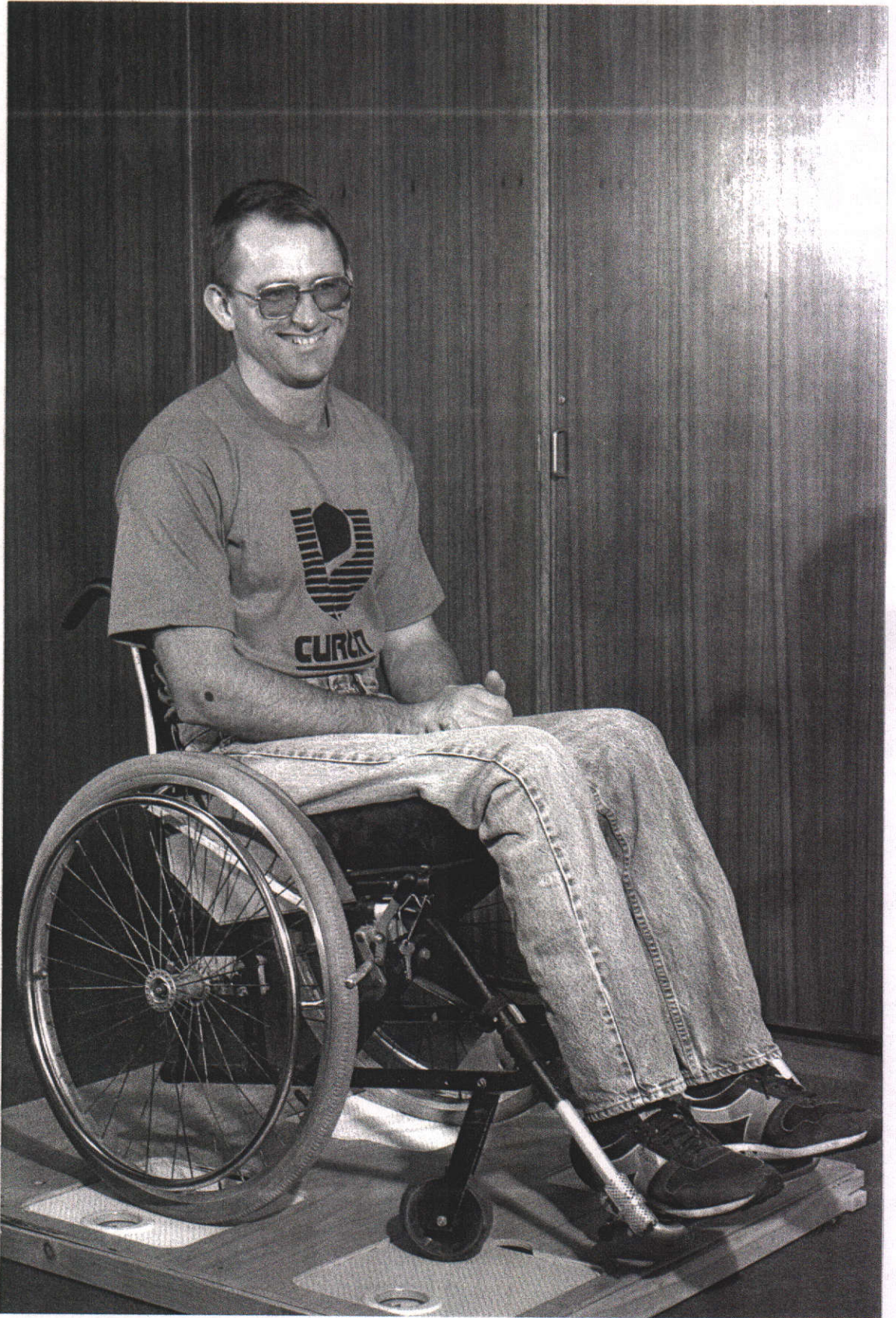
Figure 2.10 Measurement of body weight of paraplegic subjects while seated in their own wheelchair.
