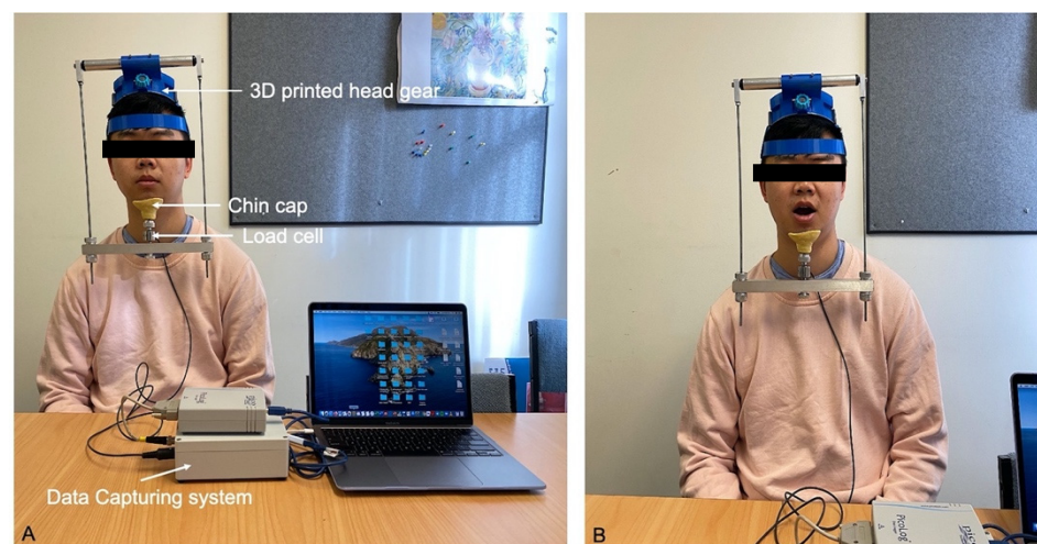
Figure 1. (A) Jaw-opening device consisting of a 3D-printed headgear, load cell, and chin cap connected to a data capturing system. (B) During maximum opening.
