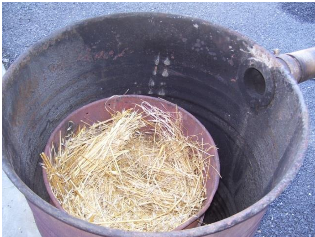
Figure 3.2 Inner fuel drum loaded with wild oats fuel and positioned in outer steel drum.
