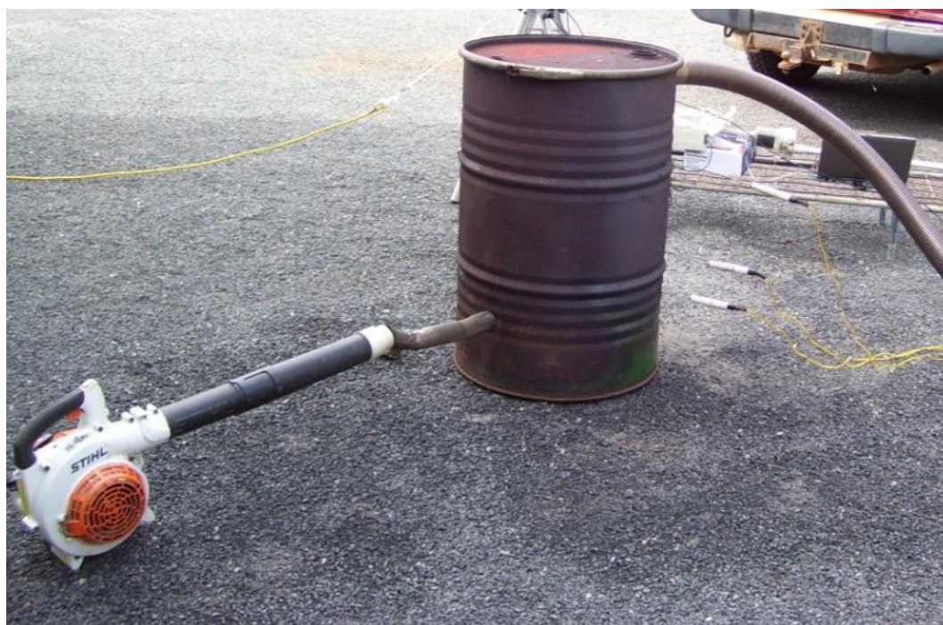
Figure 3.3 Assembled pyrolysis chamber with Stihl leaf blower, K type thermocouples and flexible steel smoke outlet.
