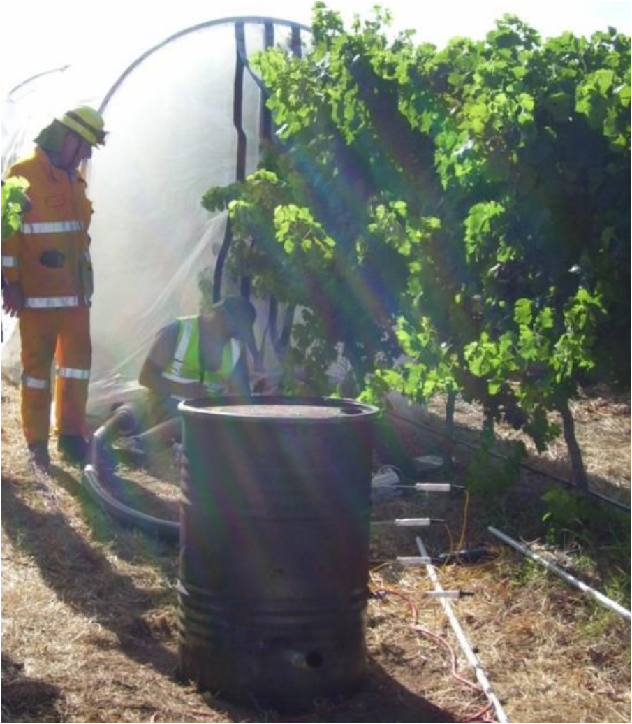
Figure 4.2 Vineyard trial with Solarweave tent and pyrolysis chamber.
