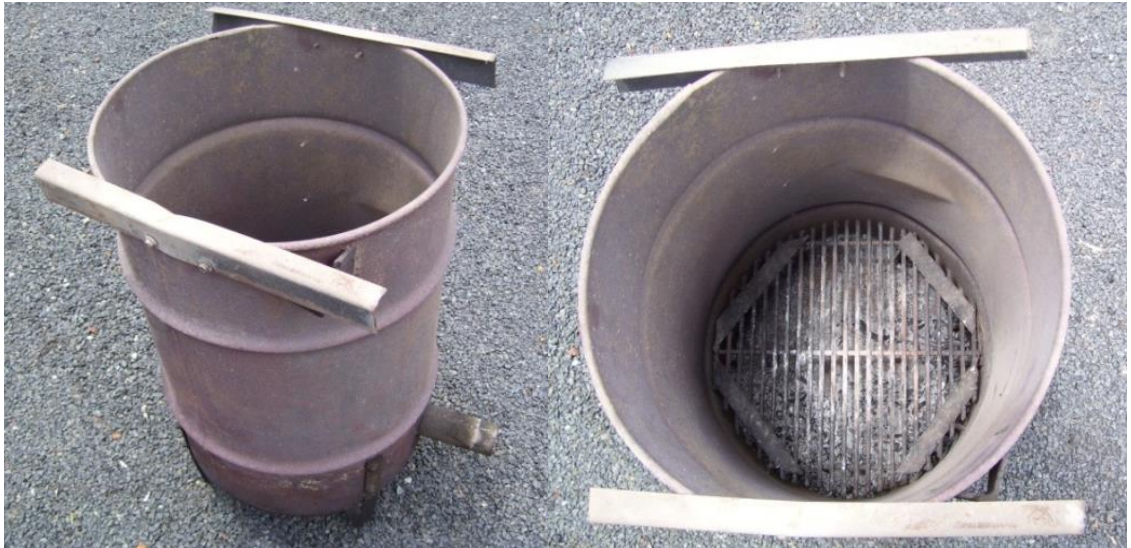
Figure 3.1 Inner fuel drum with fuel mesh screen and air inlet.
