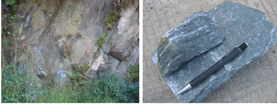
a. Outcrop of the greenschist (No. 15) b. Quartz and calcite veins in greenschist (No. 69)
