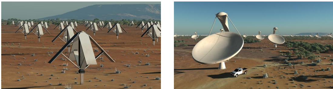
Figure 1.5: Artist impressions of the low-frequency aperture array antennas (left) and dishes with single-pixel feeds (right). Credit: SPDO/Swinburne Astronomy Productions and additionally TDP/DRAO (right).
