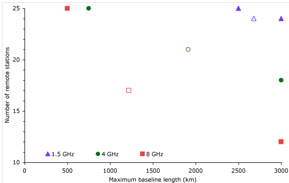
Figure 6.9: Long baseline design solutions of similar network cost, being \sim 50\% of the N_{RSt} = 25 , b_{max} = 3000 km and 8 GHz beam-bandwidth design solution. Each marker represents a design solution. The open markers are for subsets of the N_{RSt} = 25 , b_{max} = 3000 km distribution, the filled markers are for b_{max} = 3000 km or N_{RSt} = 25 .
