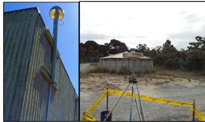
Figure 2: CUTA (Left) and CUTT (Right) GNSS antennas, baseline distance 964 m.
