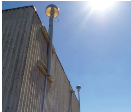
Figure 3. Curtin CUTA (Left) and CUT0 (Right) GNSS antennas used.
