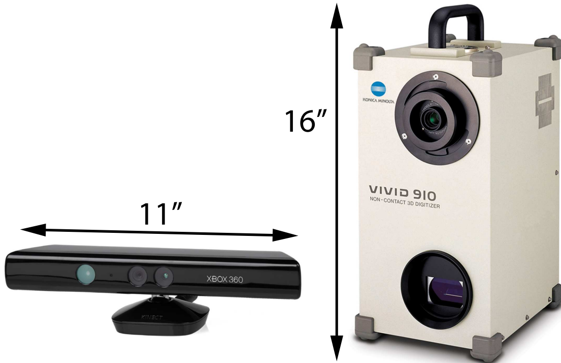
Figure 6.1: The Kinect Sensor (left) used in this work. The Minolta VIVID 910 3D scanner (right) used in FRGC.
