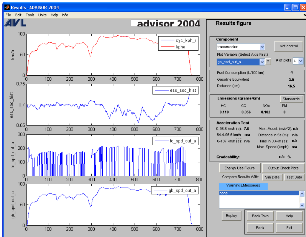
Figure A.36 - Results of the Hyundai Sonata Hybrid 2011 model for the HWFET. Measured data indicates that fuel consumption is 4.048 L/100km.
