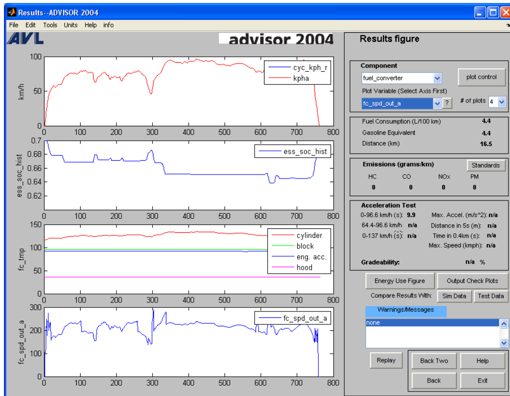
Figure A.68 - Results of the Honda CR-Z model for the HWFET. Measured data indicates that fuel consumption is 4.48 L/100km.
