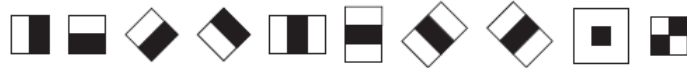
Figure 2.11: Haar features: black and white areas denote the negative and positive weights, respectively.
