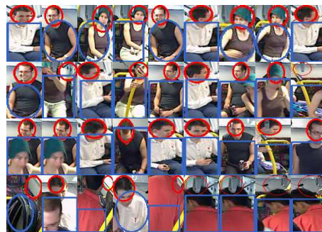
Figure 3.17: The detected passengers in video 8. The different thickness of the ellipses represent the likelihood of the human detection model (thin = low likelihood, thick = high likelihood).
