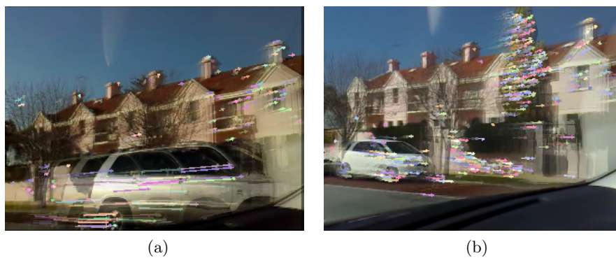
Figure 6.7: Example of two scenes with objects of different velocity. (a) A moving car has longer motion fields compared to other objects in the scene such as houses and trees. (b) Static objects normally have similar average velocity.
