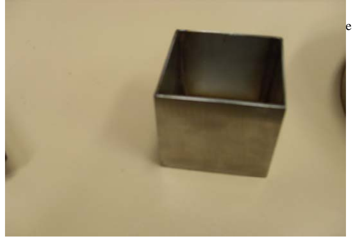
Figure 2. Metal Container used for shrinkage test
