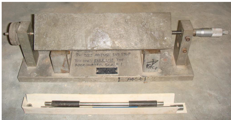
Figure 3-12: Length of drying shrinkage specimen being measured by a horizontal length comparator.
