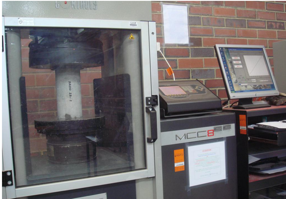
Figure 3-9: Compressive strength test machine with a sample under loading.
