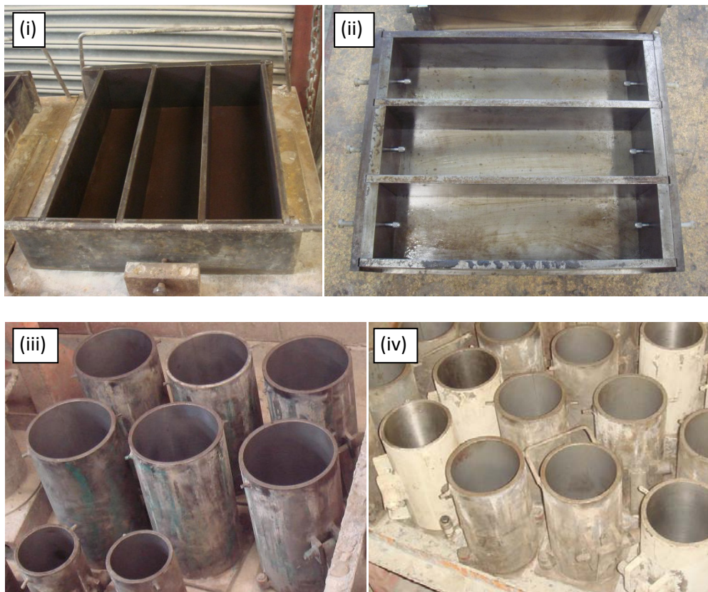
Figure 3-4: Different types of moulds: (i) flexural strength test mould, (ii) drying shrinkage test mould, (iii) tensile strength test mould and (iv) compressive strength test mould
