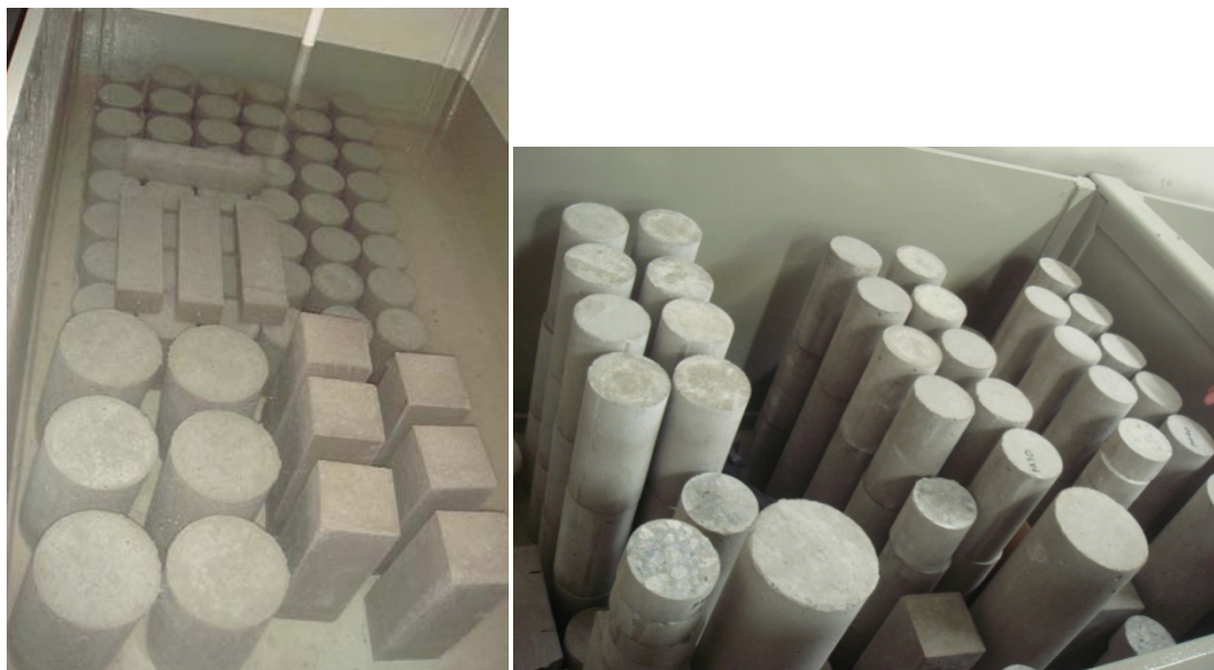
Figure 3-7: Samples cured in curing tanks (left) and in the curing room (right)
