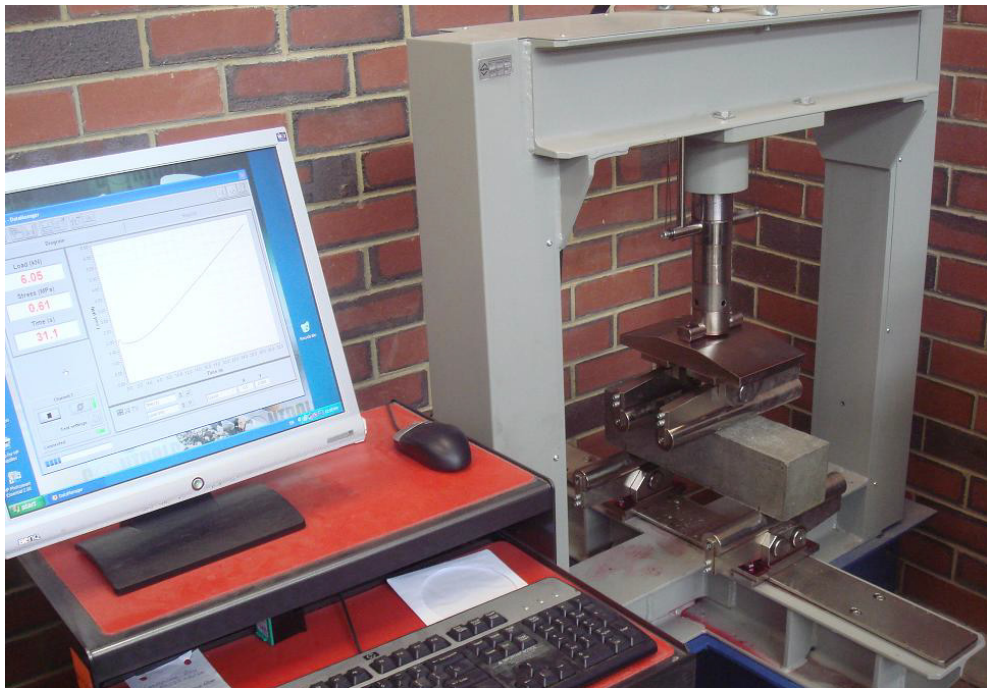
Figure 3-11: Flexural strength test in progress
