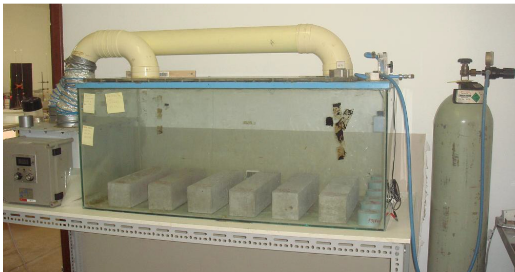
Figure 3-19: Carbonation chamber with specimens inside
