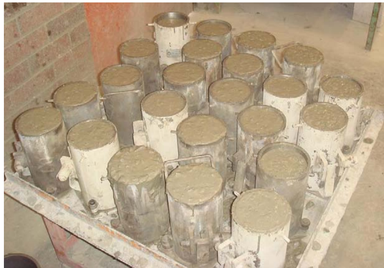
Figure 3-6: Moulds on the vibration Table
