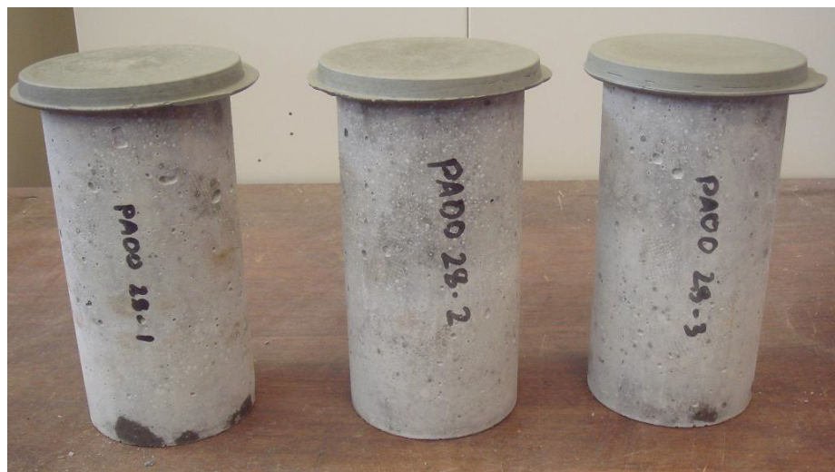
Figure 3-8: Compressive strength test specimens after sulphur capping
