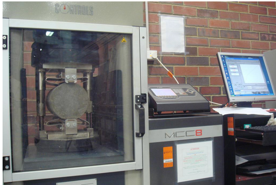
Figure 3-10: Indirect tensile strength test in progress
