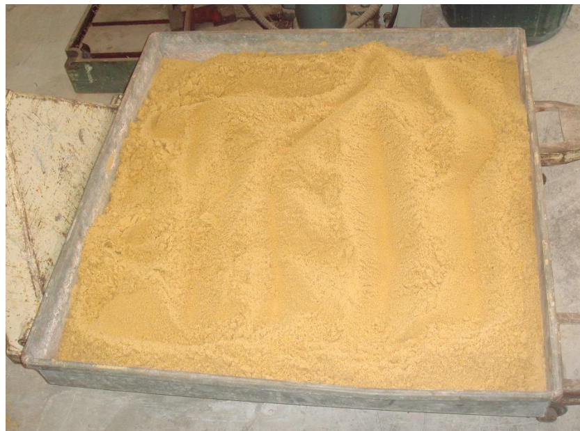
Figure 3-3: Preparation of fine aggregate for SSD condition.
