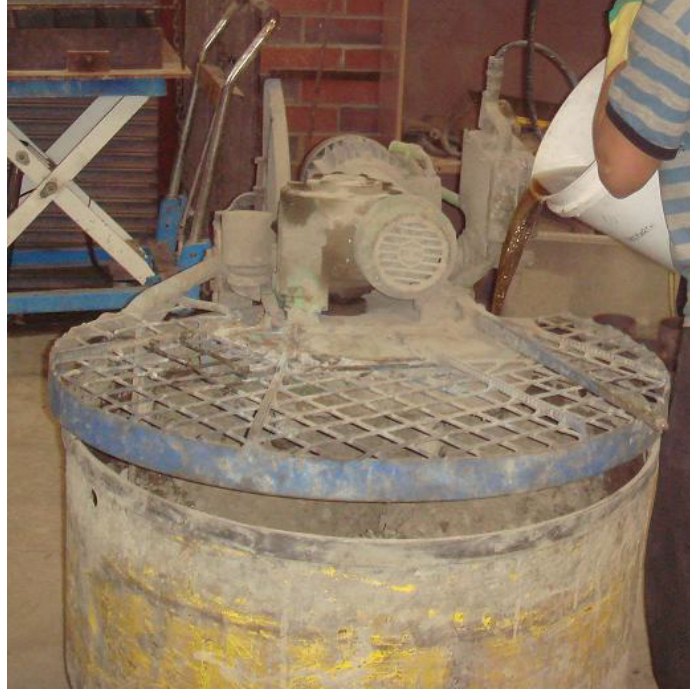
Figure 3-5: Water mixed with superplasticiser is being added in the running mixer.
