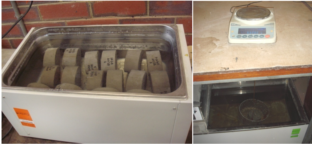
Figure 3-13: VPV samples left in water bath for cooling (left) and weighed under water (right)
