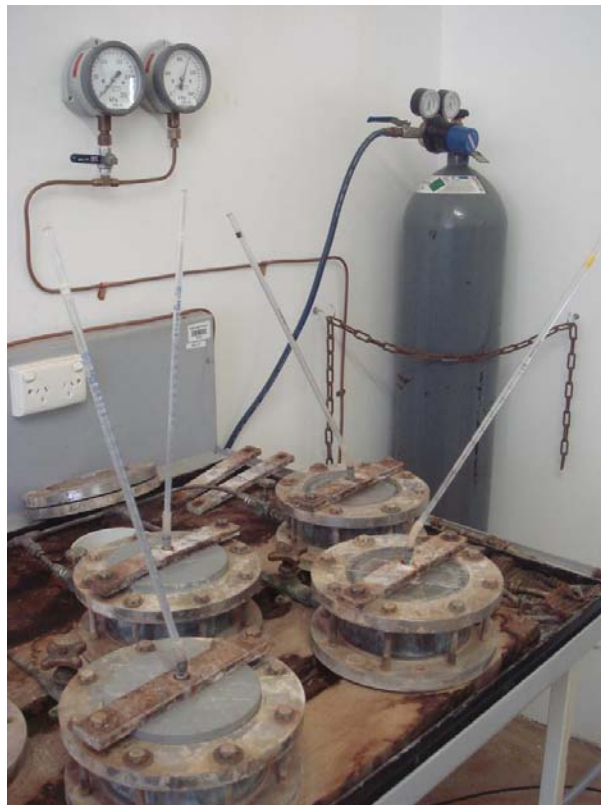
Figure 3-16: Water permeability test arrangement.
