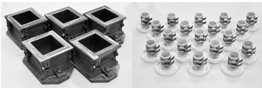
Figure 4. 10 cm cube (left) and cylindrical moulds (right) used for casting the samples.
