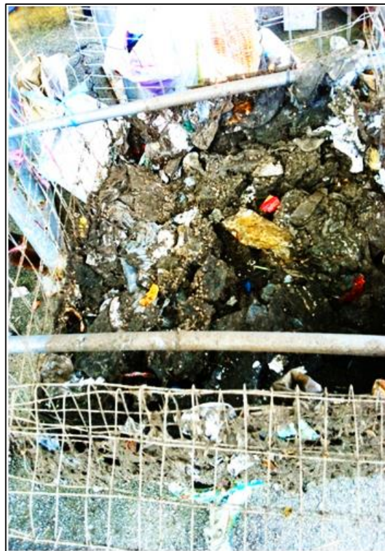
Figure 3.1 Garbage strained out from the raw septage upon the truck arrival at the project site
