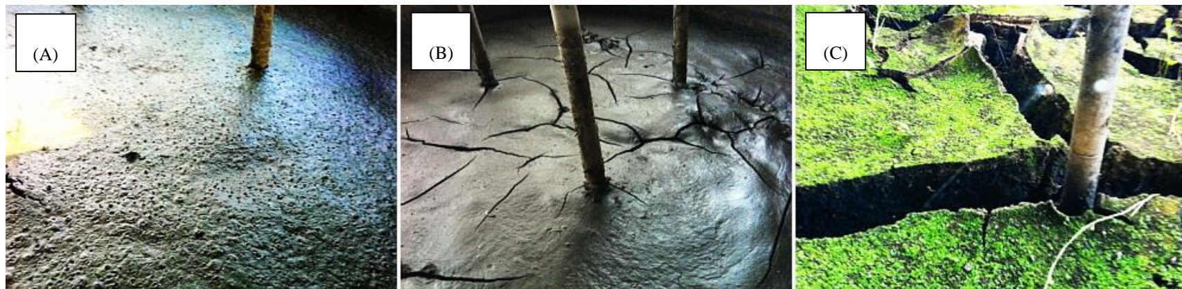
Figure 7.2 Septage deposit in unplanted wetland A2-350UP at (a) 4 days (b) 7 days (c) 30 days after septage loading under SLR 350 kg TS/m 2 /yr
