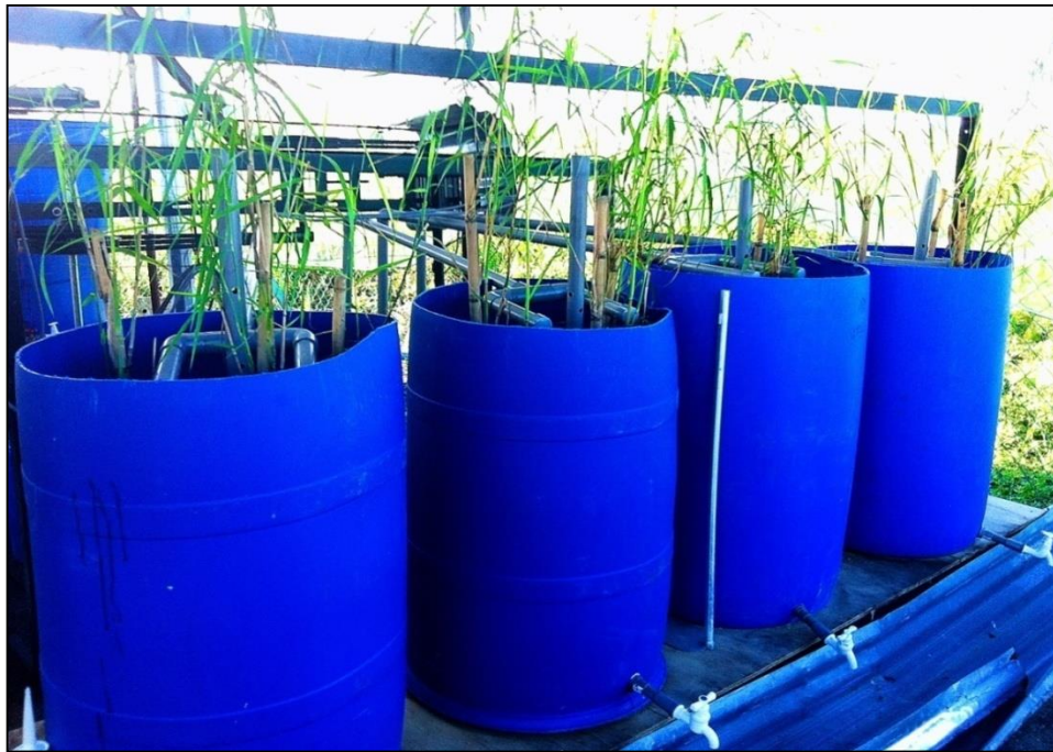
Figure 3.8 Second stage of wetlands planted with Phragmites karka completed with pipe network for septage distribution (Wetland B1-B4)
