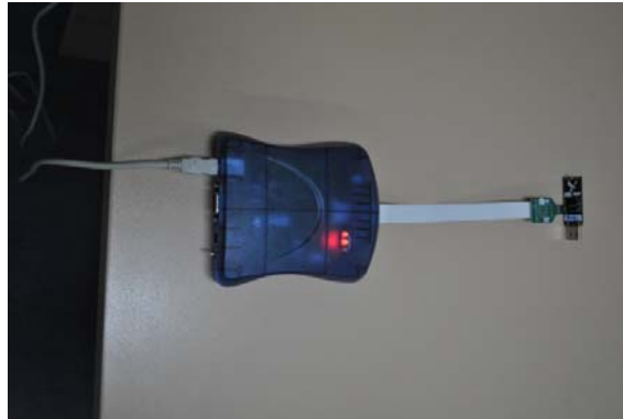
Figure 7-2: Programming RZ RAVEN USB by Atmel JTAGICE mkII
