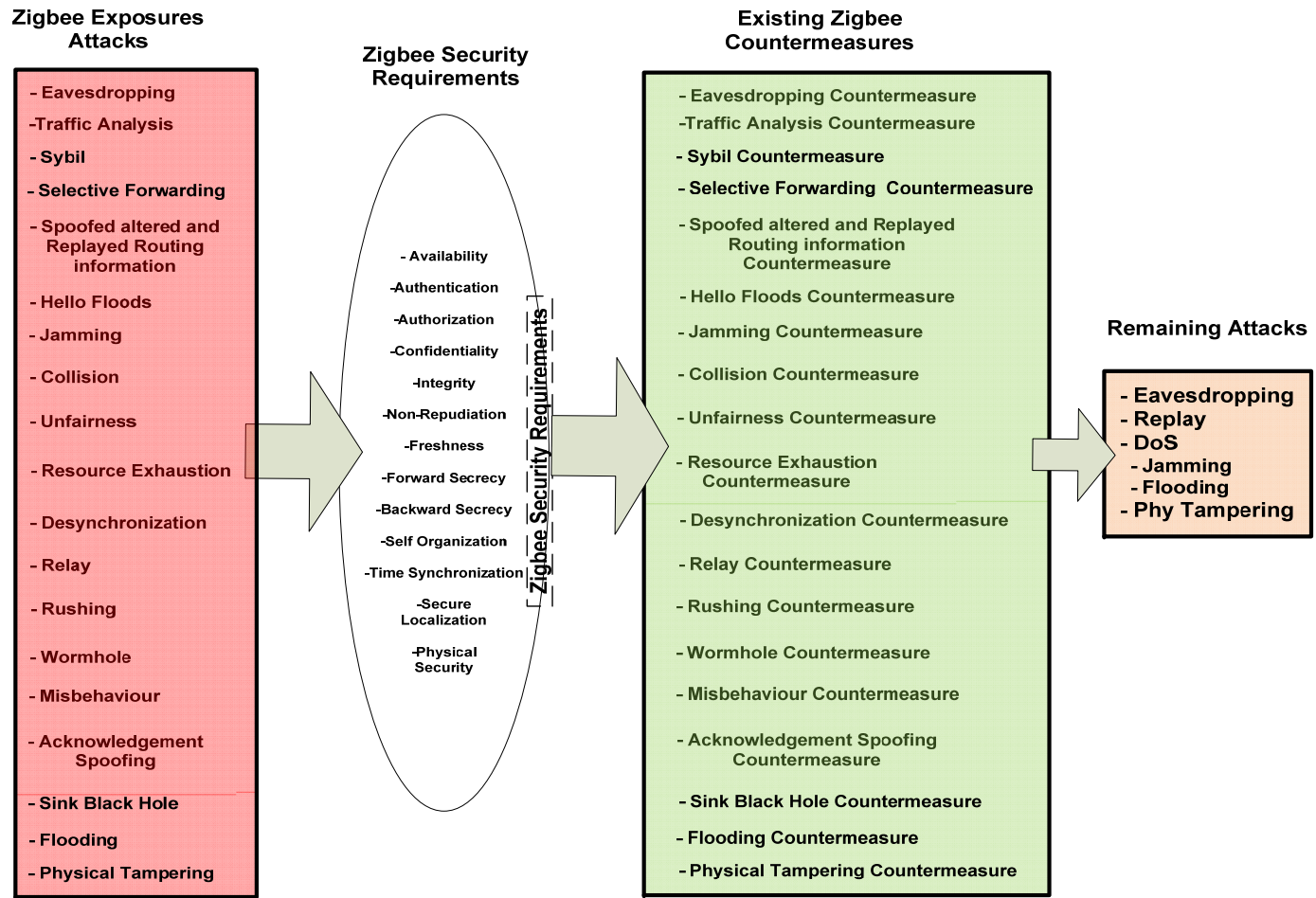
Figure 4-1: The process of Attacks Filtering
