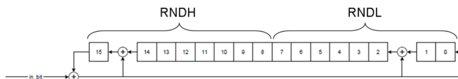
Figure 7-19: The Random Number Generator structure
