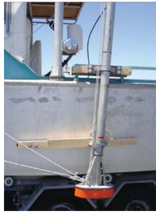
Figure 3.2.1. Pole mounting of the Simrad EQ60 single-beam echosounder on port side of the RV Snipe . Mounting is shown with pole retracted.
