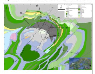
Figure 1: Geological map (modified from GTK) of the Kevitsa Ni-Cu-PGE deposit, showing locations of the previous 2D seismic profiles (E2-E5) and the 3D survey area (boxed area).
