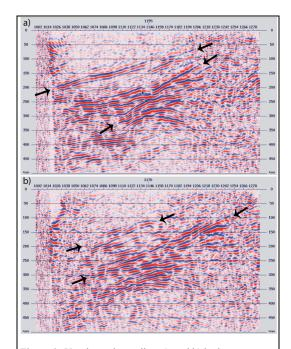
Figure 6: Unmigrated crosslines (a and b) in the eastern part of the seismic cube, clearly showing a series of gently and steeply dipping reflections and even diffractions.
