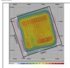
Figure 2: CDP fold coverage, shots and receiver locations of the Kevitsa 3D survey.
