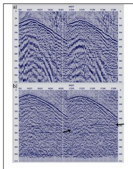
Figure 3: An example shot record (shown for two reciver lines) before (a) and after (b) various processing steps. Note the increase in the signal quality in (b) and specially the reflection marked by the arrows.
