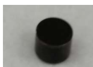
Figure 3.6: Photograph of GC stub (5 mm diameter) used for electrochemical experiments.
