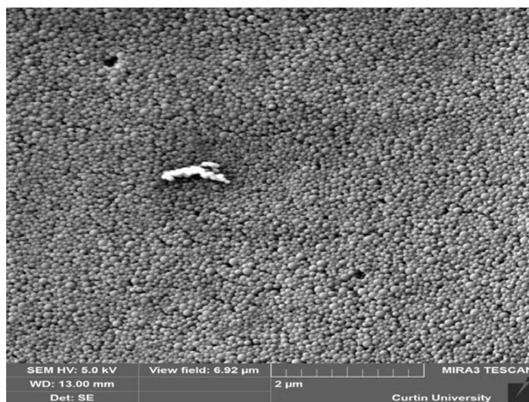
Figure 9.2: Scanning electron micrograph of 100 nm polystyrene beads on a glassy carbon electrode surface.
