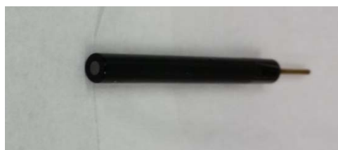
Figure 3.10: Photograph of macroelectrodes used for electrochemical experiments purchased from BASi
