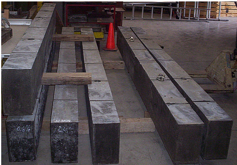
Figure 3.7 Beams after Demoulding
