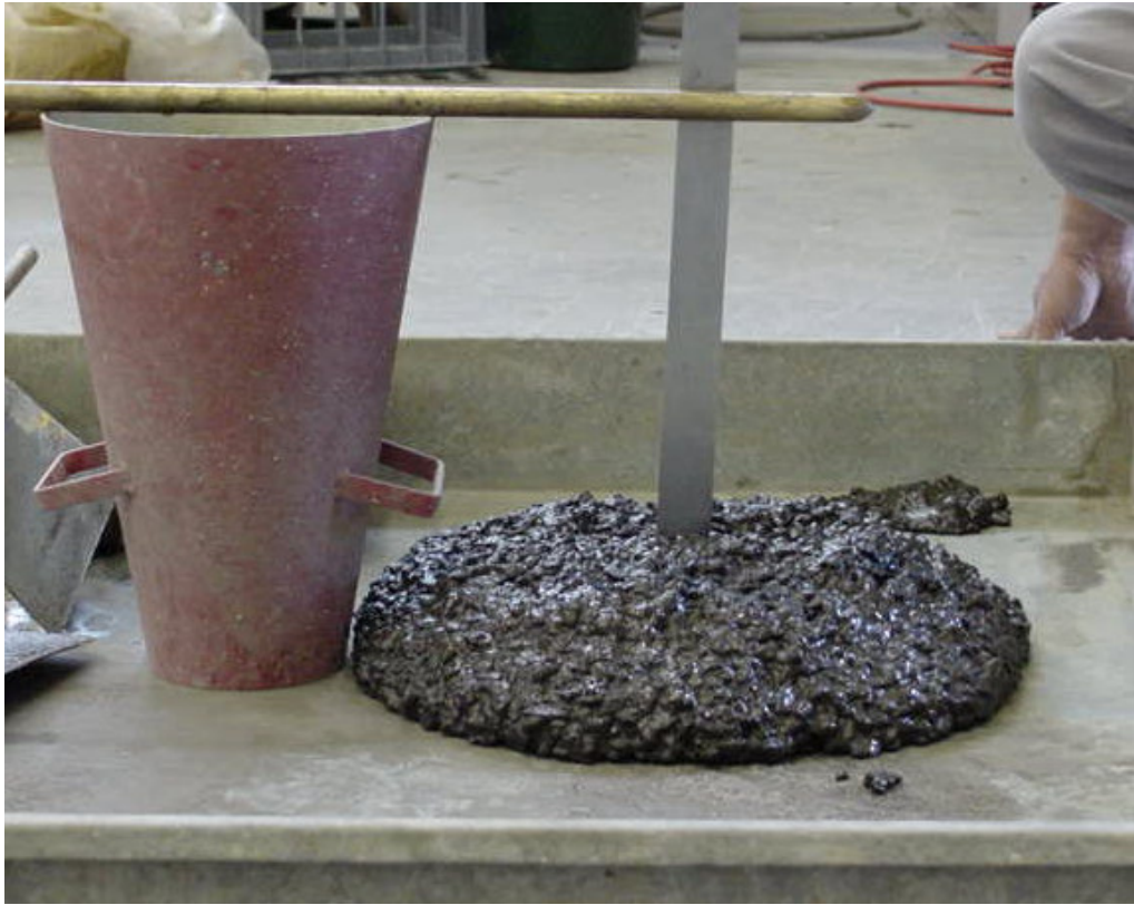
Figure 3.10 Slump Test of Fresh Concrete
