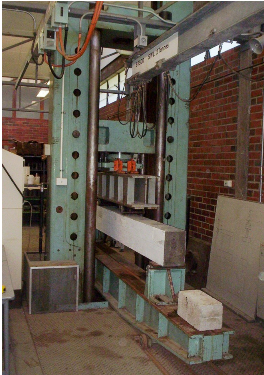
Figure 3.9 Beam Test Set-up
