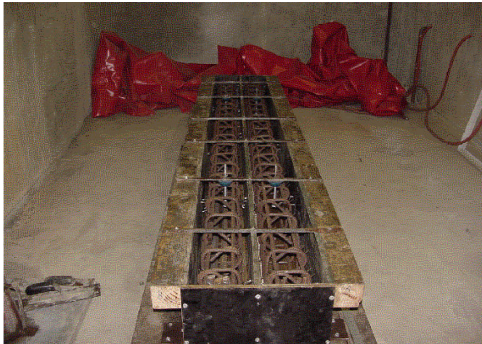
Figure 3.3 Moulds with Reinforcement Cages
