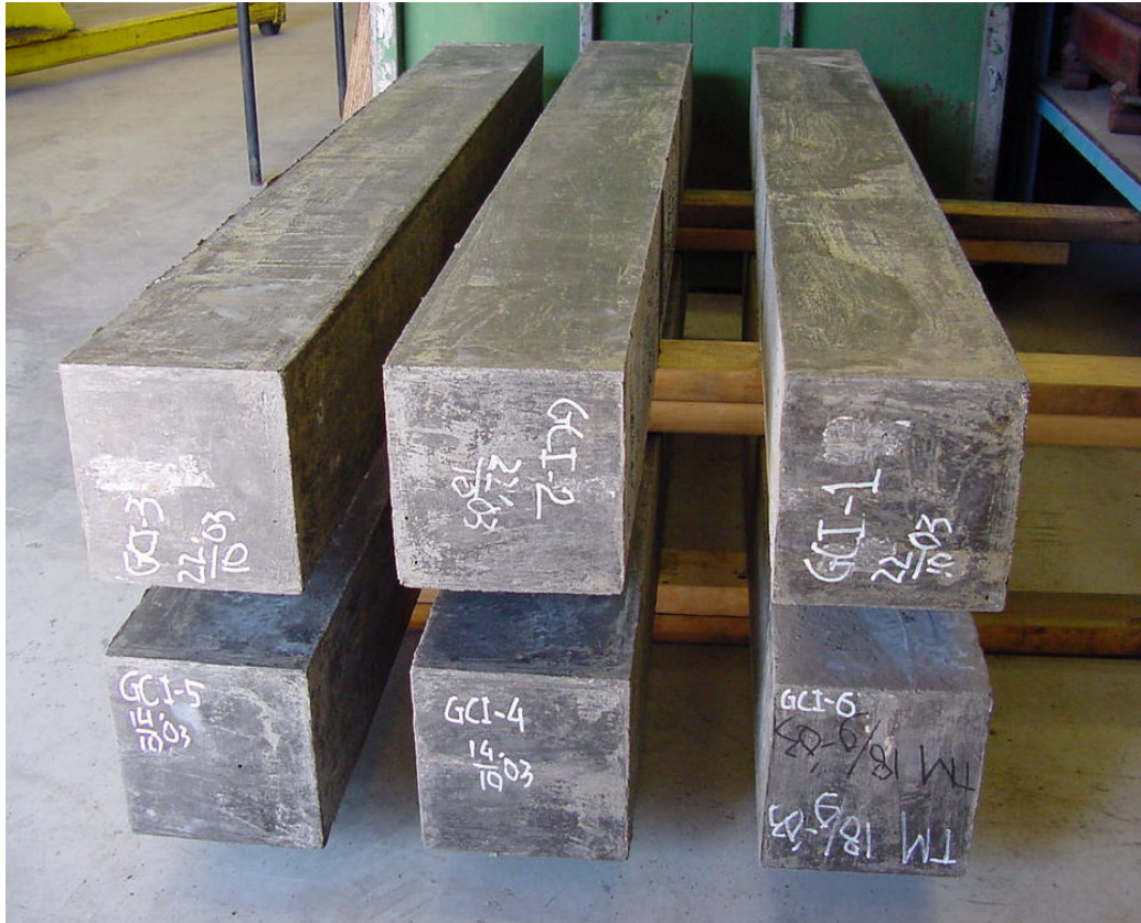
Figure 3.14 Columns after Demoulding
