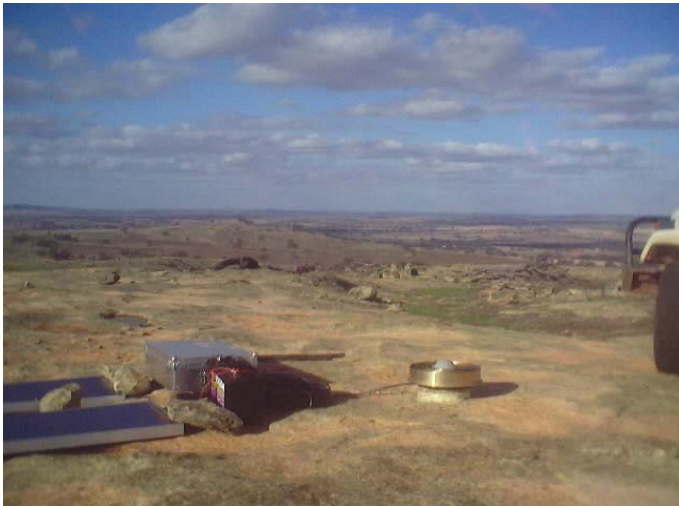
Figure 3. The GPS receiver was powered by a combination of solar panels and car batteries and left unattended (excepting checks) during each site occupation.
