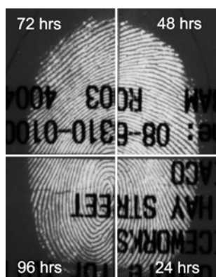
Fig.4 Latent fingermark on printed thermal paper where quarters were treated for different development times with fluorous acid-free/IND/ZnCl 2 by the dry contact method. Photographs were taken using a Nikon D100 Camera in luminescence mode with settings; Focal length: 85 mm, Shutter Speed: 2.5 s and Aperture: f/11.
