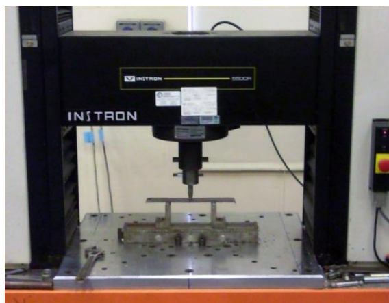
Figure 3: Flexural testing being conducted
