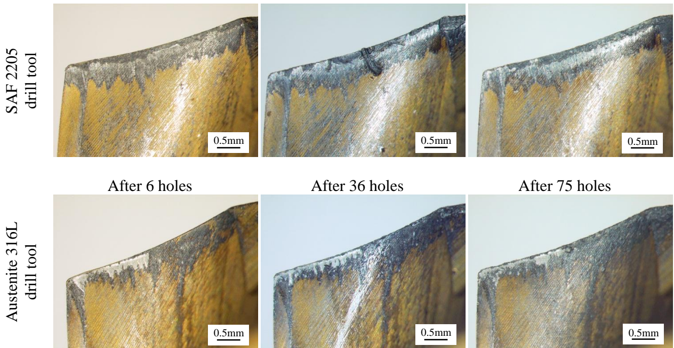
Fig. 7 Micrograph images of the rake face of drill tools during the progression of drilling trials.
