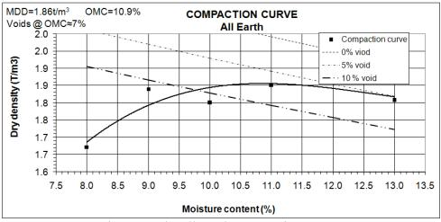
Figure 2: The all Earth compaction curve.
