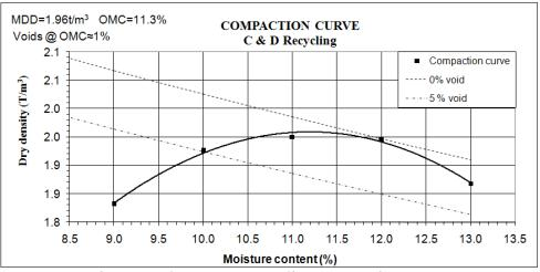
Figure 1: The C & D Recycling compaction curve.
