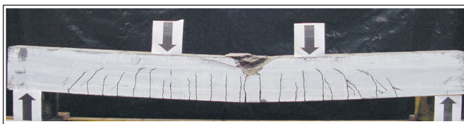
Figure 9. Crack Pattern and Failure Mode of Reinforced Geopolymer Concrete Beam [13]
