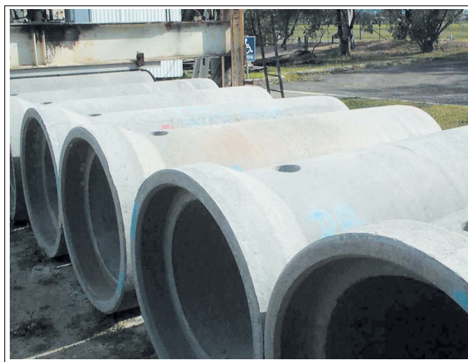
Figure 12. Geopolymer Concrete 1500 mm Sewer Pipes [8]
