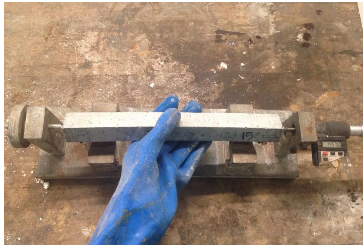
Figure 3. Length measurement of a mortar bar specimen.
