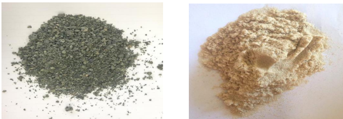
122 Figure 1. Granulated FNS (left) and natural sand (right).
