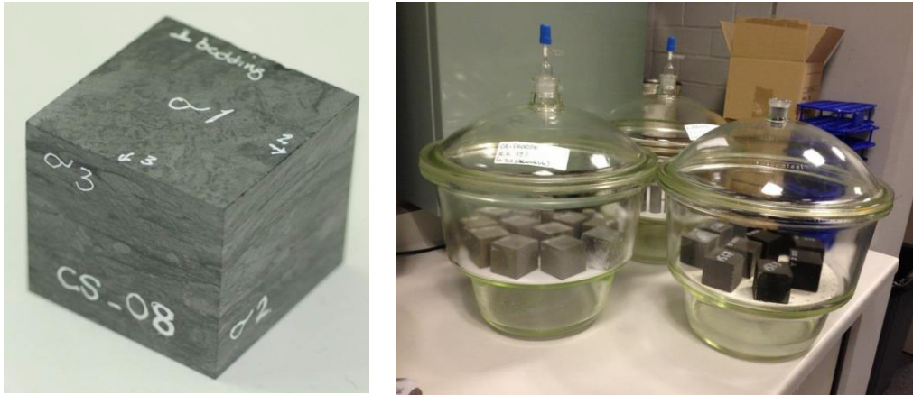
Figure 13: Carynginia cubic sample (left) and relative humidity environments established in glass desiccators for saturation of samples
