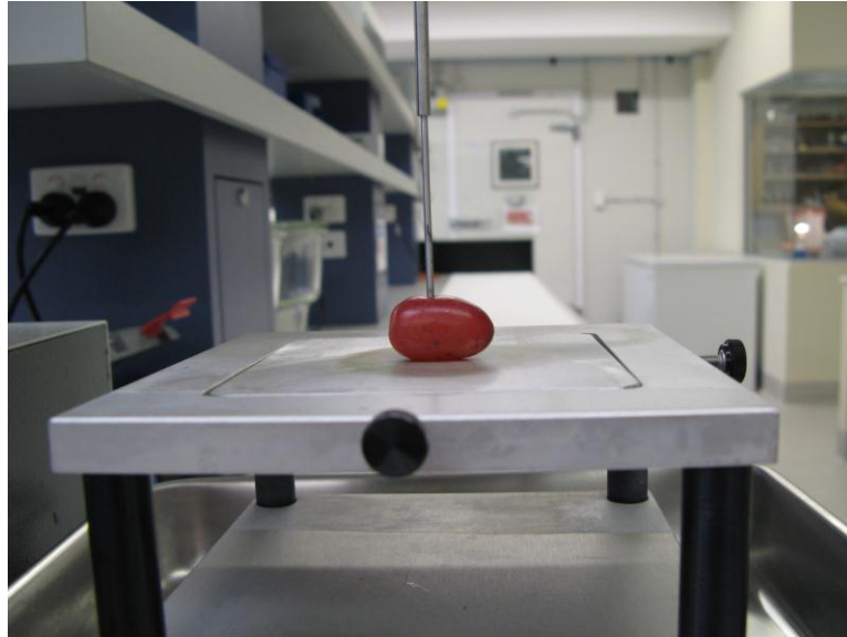
Figure 3.3 Grape puncture test using texture analyser.
