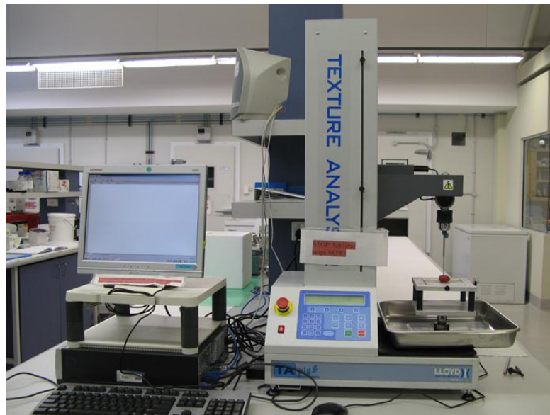
Figure 3.2 Texture analyser linked to personal computer with Nexygen ® software.
