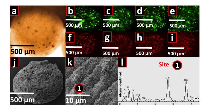
Figure 2: Micrographs of F2 (control) microcapsules. a: optical image of F2, b-e: confocal images of CFSE stained cells within F2 microcapsules, f-i: confocal images of fluorescent labelled UDCA within F2 microcapsules, j: SEM micrograph of F2, k: surface site used for EDXR analysis, I: EDXR spectral analysis.
