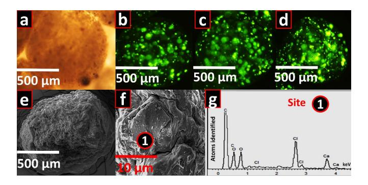
Figure 1: Micrographs of F1 (control) microcapsules. a: optical image of F1, b-d: confocal images of CFSE stained cells within F1 microcapsules, e: SEM micrograph of F1, f: surface site used for EDXR analysis, g: EDXR spectral analysis.
