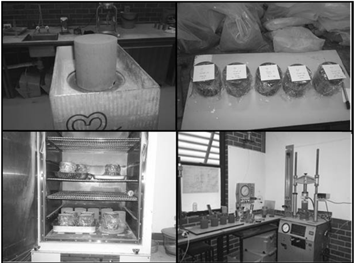
Figure 4. Sample preparation for unconfined compressive strength tests
