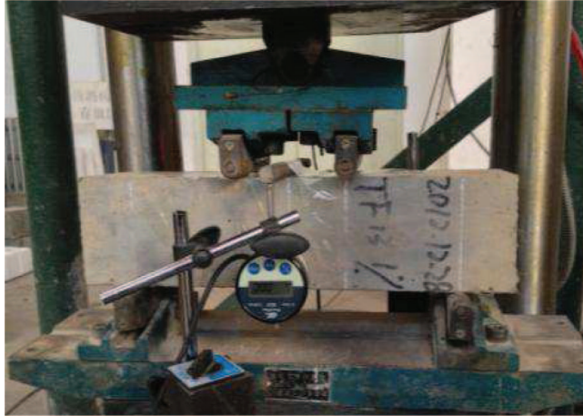
Figure 6. Setup of the flexural tensile tests
