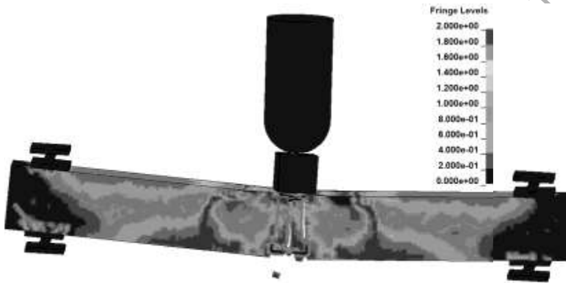
(a) Plastic strain of the RC beam after 0.1 s
