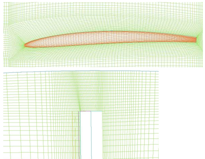
Figure 3 View of a structured grid at (a) horizontal plane crossing the blade tip and (b) cross section plane located at the blade centre.
