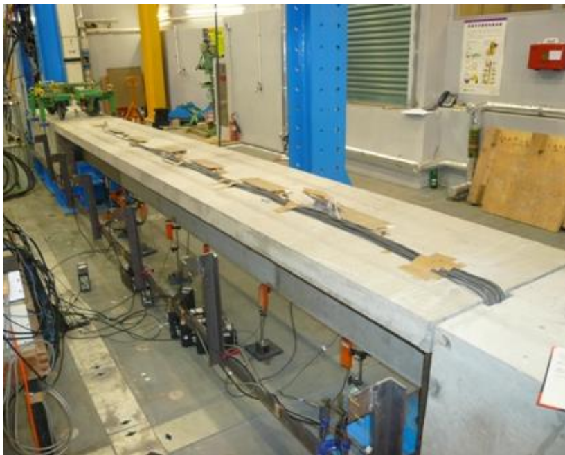
(b) Optical triggers and accelerometers
