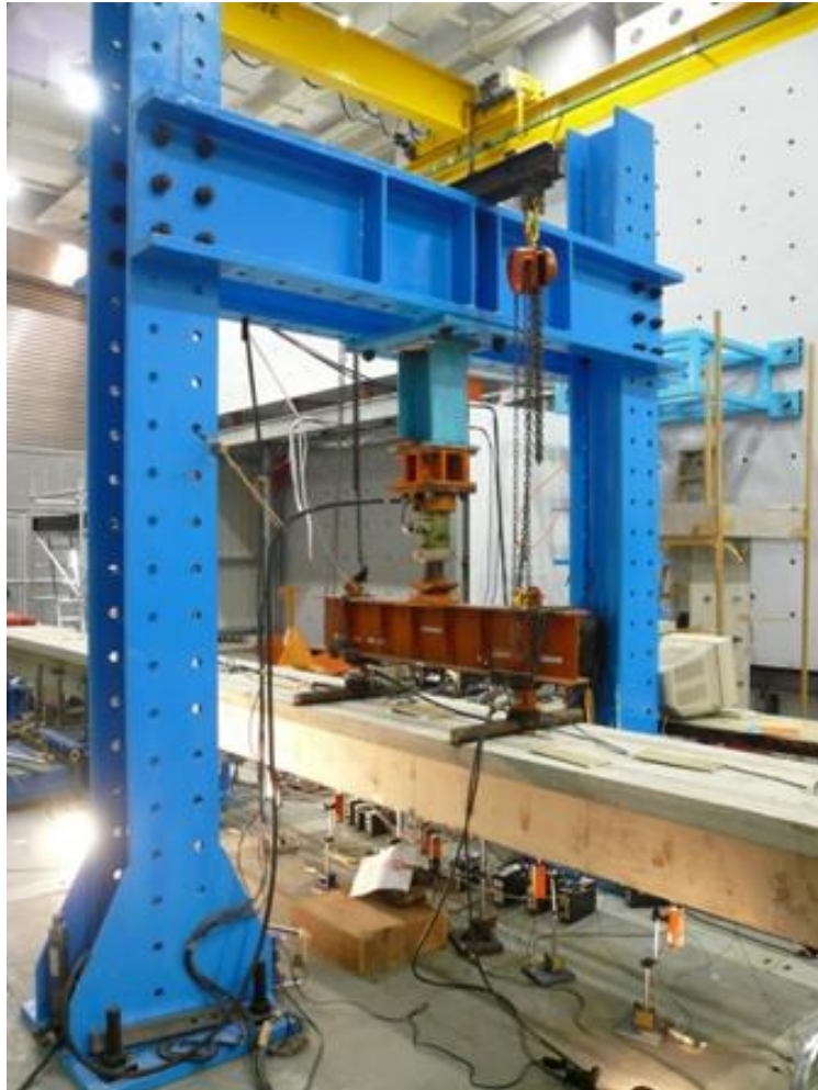
Figure 12 – Application of static load to the beam
