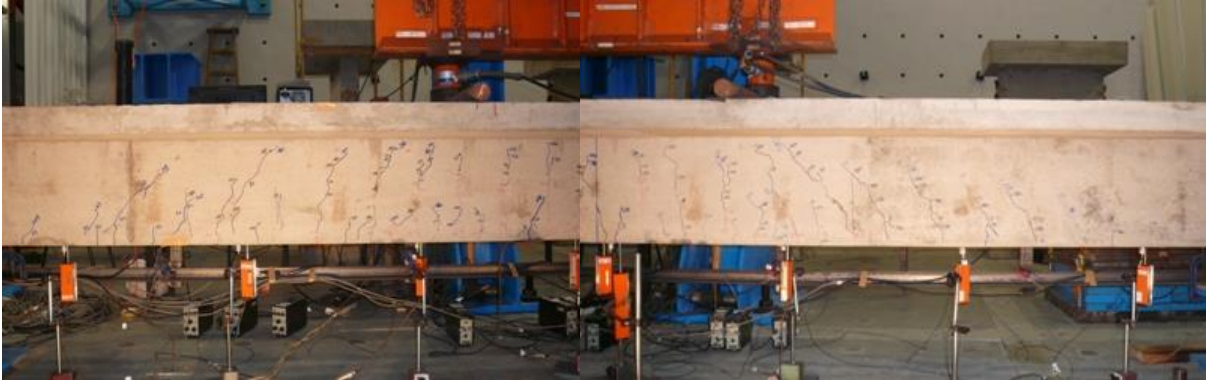
Figure 13 - Observed crack pattern in web elements of the beam
