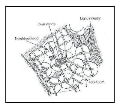
Figure 1 – District-level design schematic
