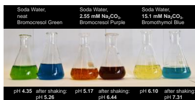
Figure 1. Photograph of soda water containing different amounts of added sodium carbonate to adjust the initial pH without (left flasks) and after (right flasks) shaking for 20 s. Traces of the pH indicating dyes were added to elucidate the pH shift.
