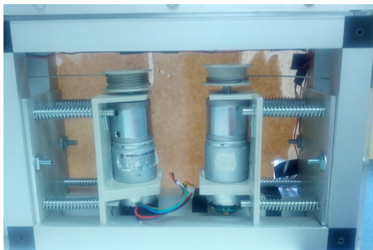
Figure 7 The antagonistic actuation
