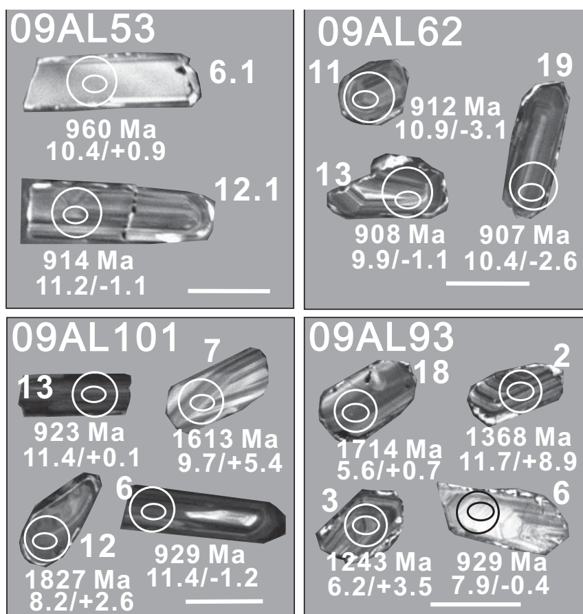
Fig. 9. Cathodoluminescence images of representative zircons for in situ analyses of U-Pb and/or Hf-O isotopes. Small ellipses indicate the SIMS analytical spots for U-Pb and/or O isotopes, and large circles denote the LA-MC-ICPMS analytical spots for Lu-Hf isotopes. Numbers near the analysis spots are the U-Pb ages (Ma) and \epsilon_{\text{Hf}}(t)/\delta^{18}\text{O} values. The white scale bars are 100 \mu\text{m} long.
