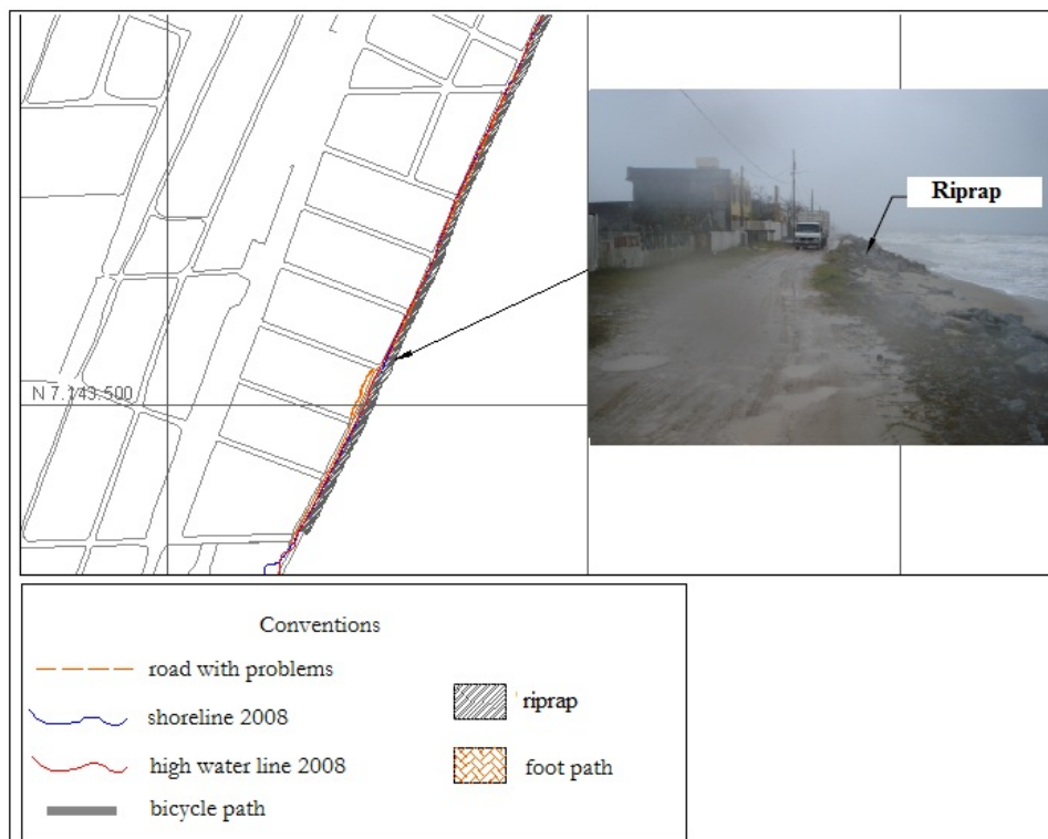
Figure 8: The part of thematic map of the study area, covering sector II.
