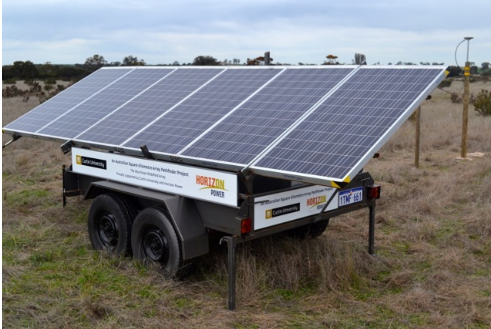
Figure 5.7: One of 3 solar power supplies constructed by the author and colleagues. This is a current deployment on the Australian Space Academy campus at Meckering and is returning data in real-time over a 3G cell connection. Electrical components were supplied courtesy of Horizon Power Pty. Ltd. Perth, W.A.
