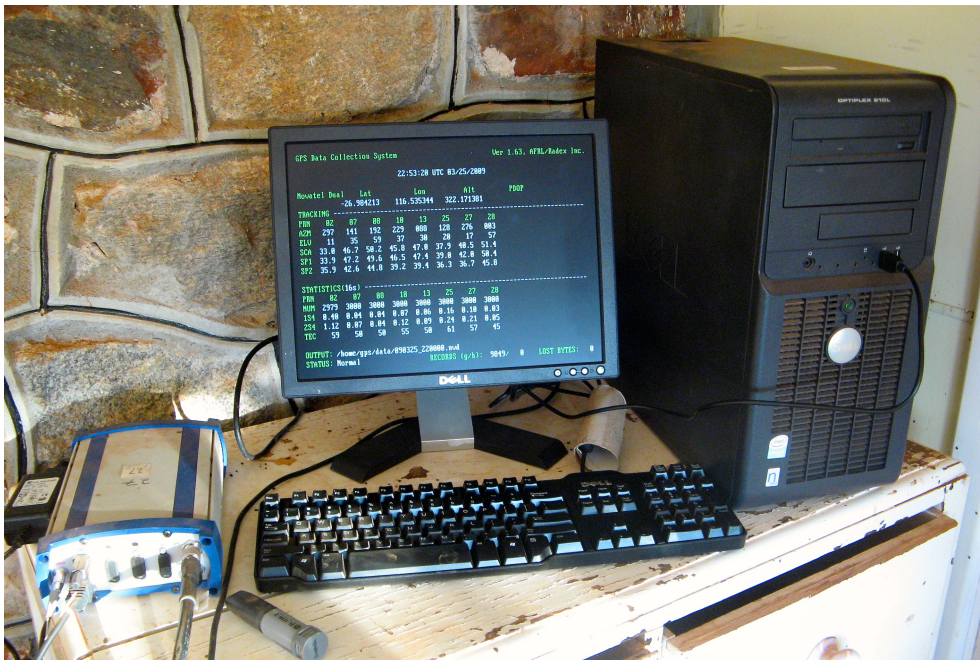
Figure 5.1: A GPS receiver, monitor and computer at Boolardy homestead in March 2009. The pencil shaped device in front of and to the right of, the receiver is a temperature logger.
