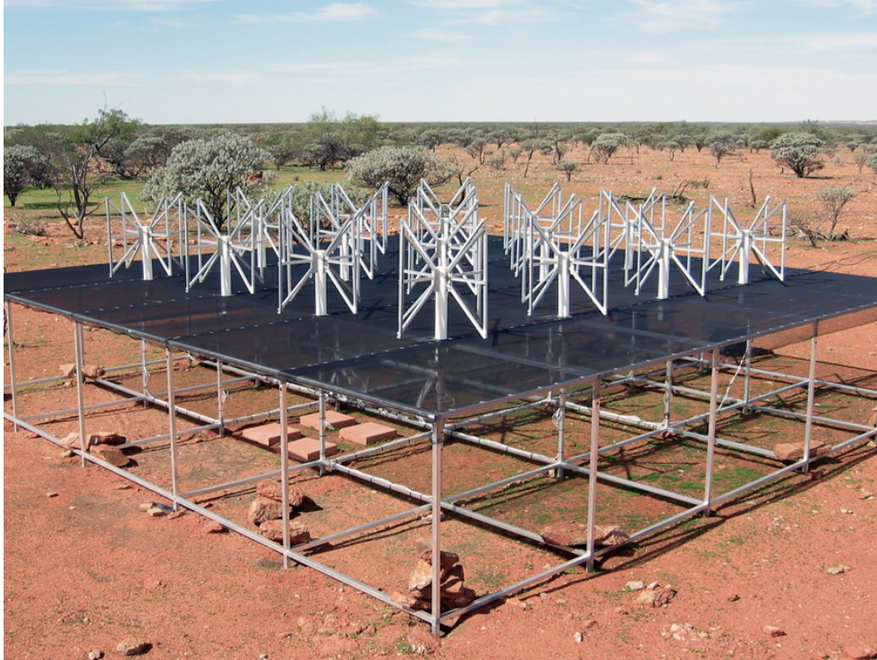
Figure 2.6: An early, prototype tile designed and fabricated by the author, housing 16 first generation antennas. (ED2 - Tile 2). Image - David Herne.
