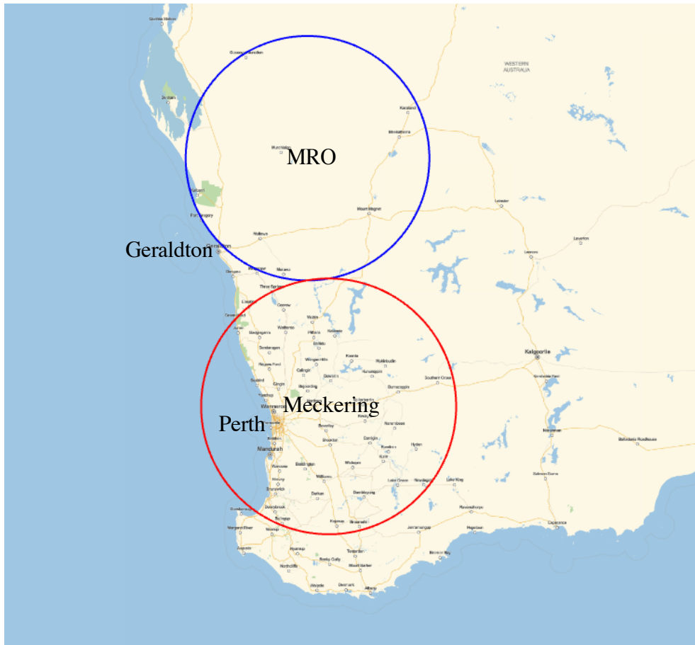
Figure 6.13: TEC observations on the MRO and at Meckering were constrained to 50° elevation, ensuring that the ionospheric observations (at 350 km altitude) by each GPS receiver didn't overlap.
