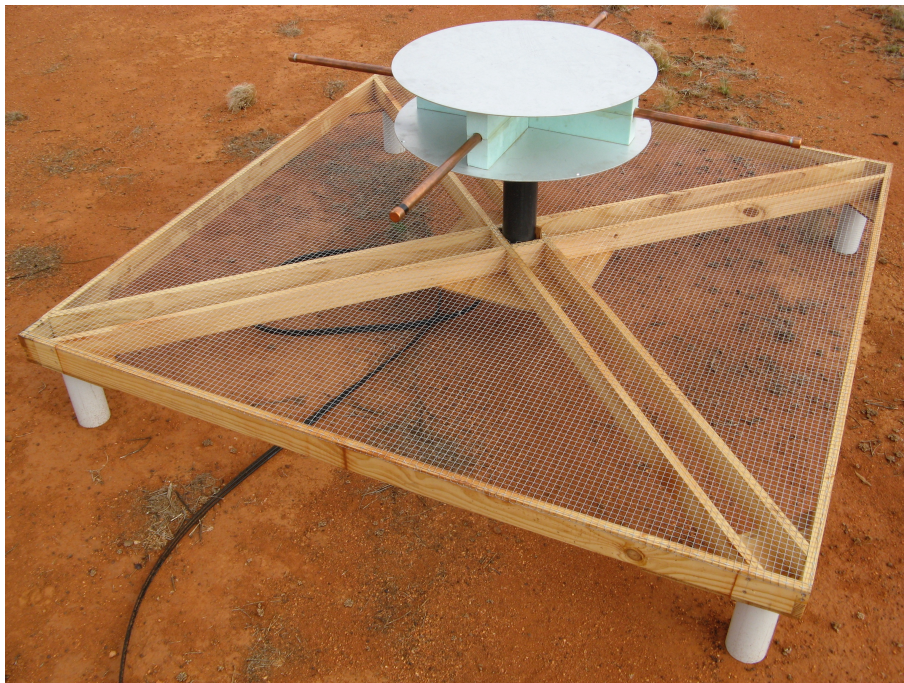
Figure 2.19: One of four PAPER ground screens designed and constructed by the author. Each mounts a single sleeved-dipole antenna.
