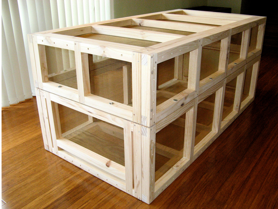
Figure 2.18: Economic, large volume EMC enclosure (Faraday cage) designed and constructed by the author following a design by Richard Bradley of the National Radio Observatory, Charlottesville, Virginia. Enclosure employed by PAPER during the field campaign (PWA-4) in July 2009 at the MRO (Figure 2.17).
