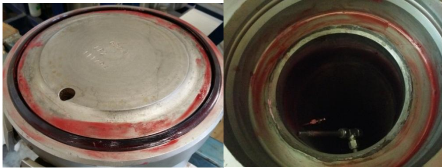
Figure 90 Closure doors and GD locks
