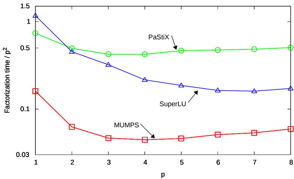
Figure 8: Execution time divided by  $p^2$  measured for parallel MUMPS, SuperLU and PaStiX solvers executed over distributed memory machine, for a two dimensional problem with  $256 \times 256$  elements, for continuity  $C^{p-1}$  for different  $p$ , one core per node, with eight nodes.
