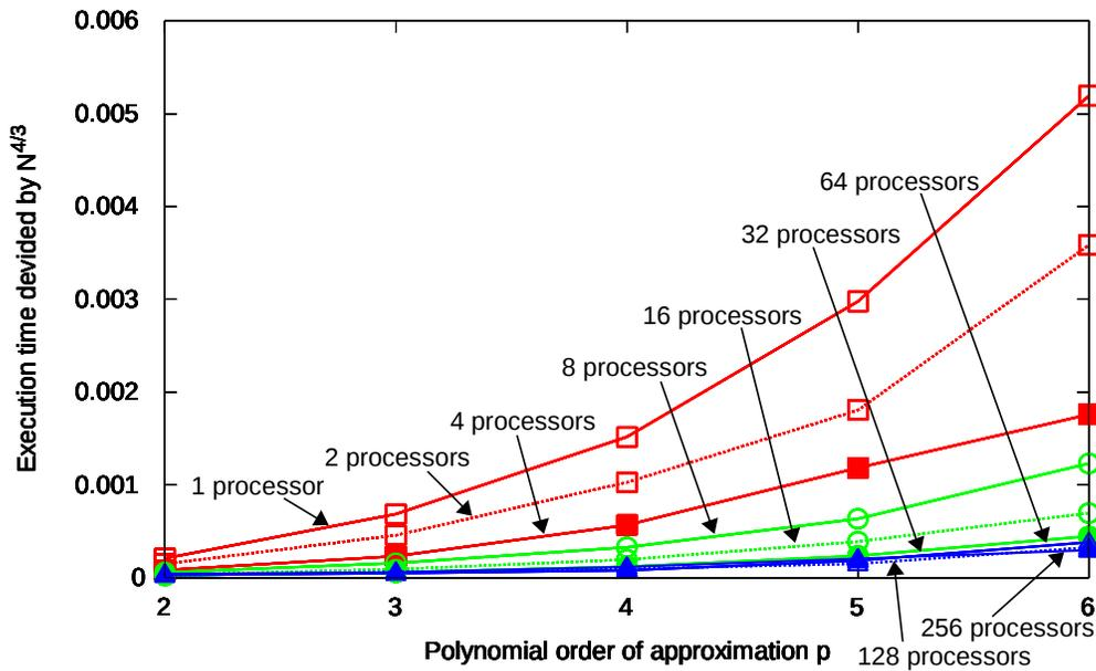
Figure 19: Execution times for the MUMPS direct solver for 3D IGA, for fixed  $32^3$  elements, divided by  $N^{4/3}$ .
