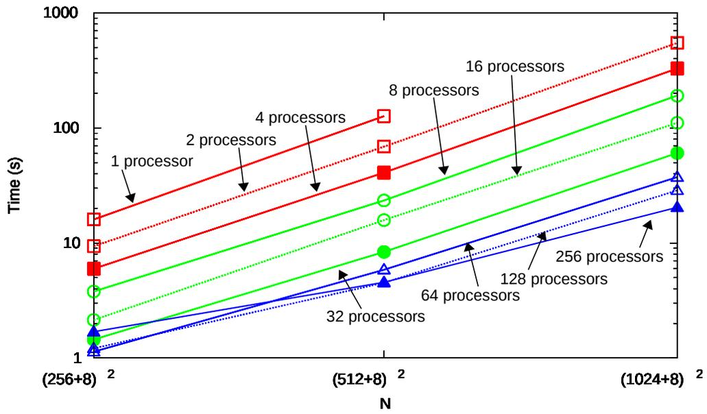
Figure 12: Execution times for the MUMPS direct solver for 2D IGA with octic B-splines,  $C^7$  global continuity.
