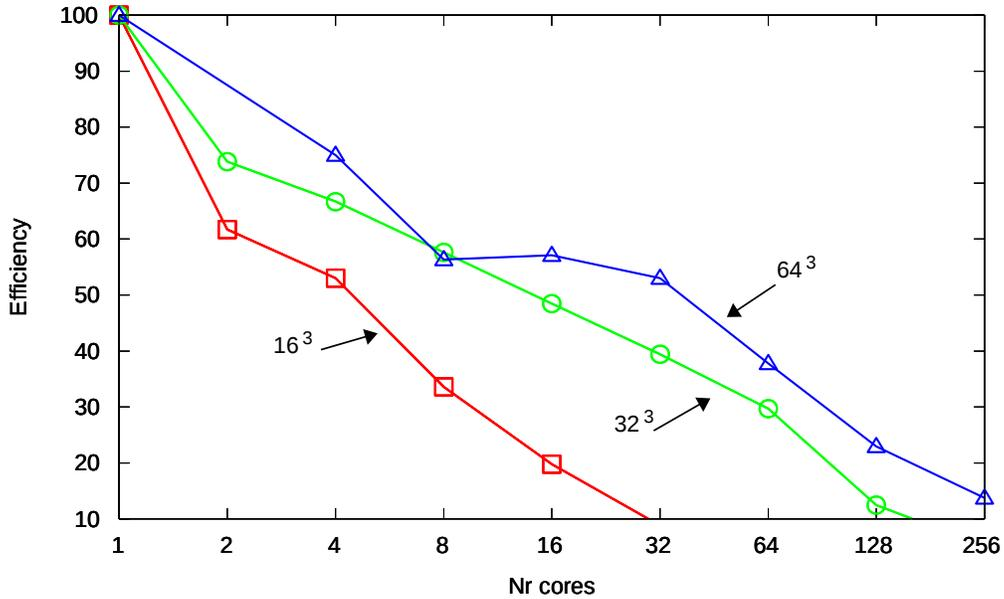
Figure 16: Parallel efficiency of the MUMPS direct solver for 3D IGA with quartic B-splines,  $C^3$  global continuity. Different plots represents different sizes of the mesh.
