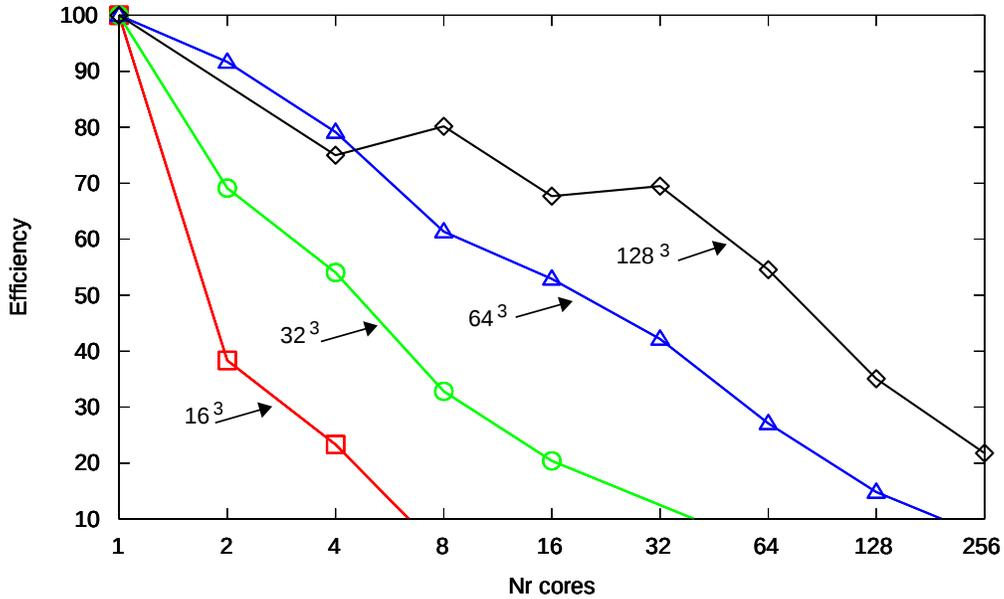
Figure 15: Parallel efficiency of the MUMPS direct solver for 3D IGA with linear B-splines,  $C^0$  global continuity. Different lines represents different sizes of the mesh.
