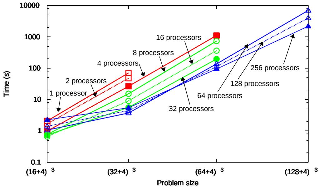
Figure 18: Execution times for the MUMPS direct solver for 3D IGA with quartic B-splines,  $C^3$  global continuity.
