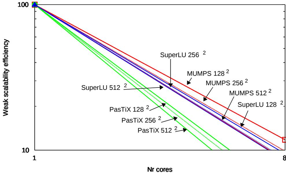
Figure 5: Weak scaling efficiency of the direct solvers for 2D IGA with quartic B-splines,  $C^3$  global continuity.
