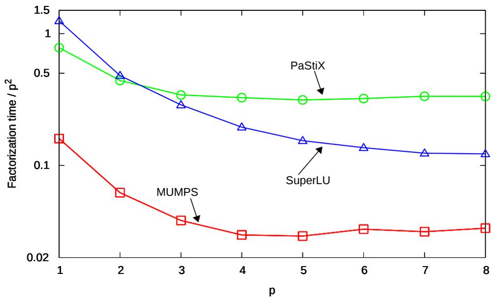
Figure 9: Execution time divided by  $p^2$  measured for parallel MUMPS, SuperLU and PaStiX solvers executed over distributed memory machine, for a two dimensional problem with  $256 \times 256$  elements, for continuity  $C^{p-1}$  for different  $p$ , one core per node, with thirty two nodes.
