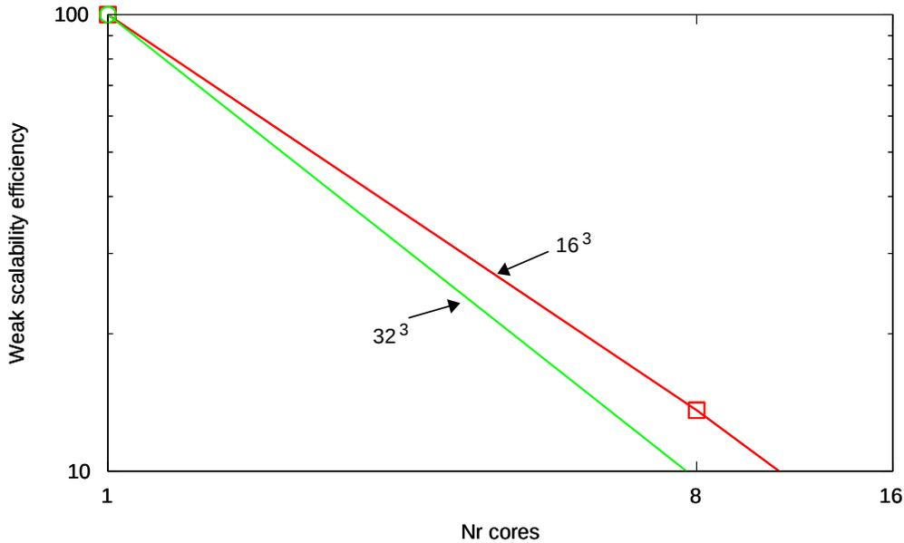
Figure 14: Weak scalability of the MUMPS direct solver for 3D IGA with quartic B-splines,  $C^3$  global continuity. Different lines correspond to various problems sizes.
