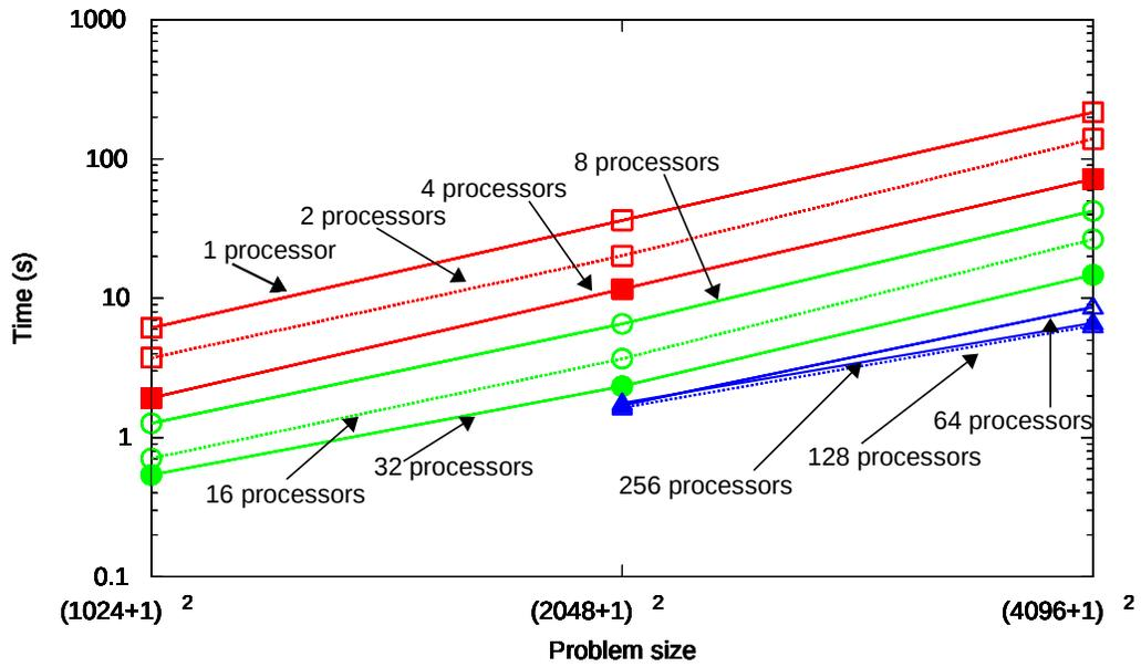
Figure 10: Execution times for the MUMPS direct solver for 2D IGA with linear B-splines,  $C^0$  global continuity.
