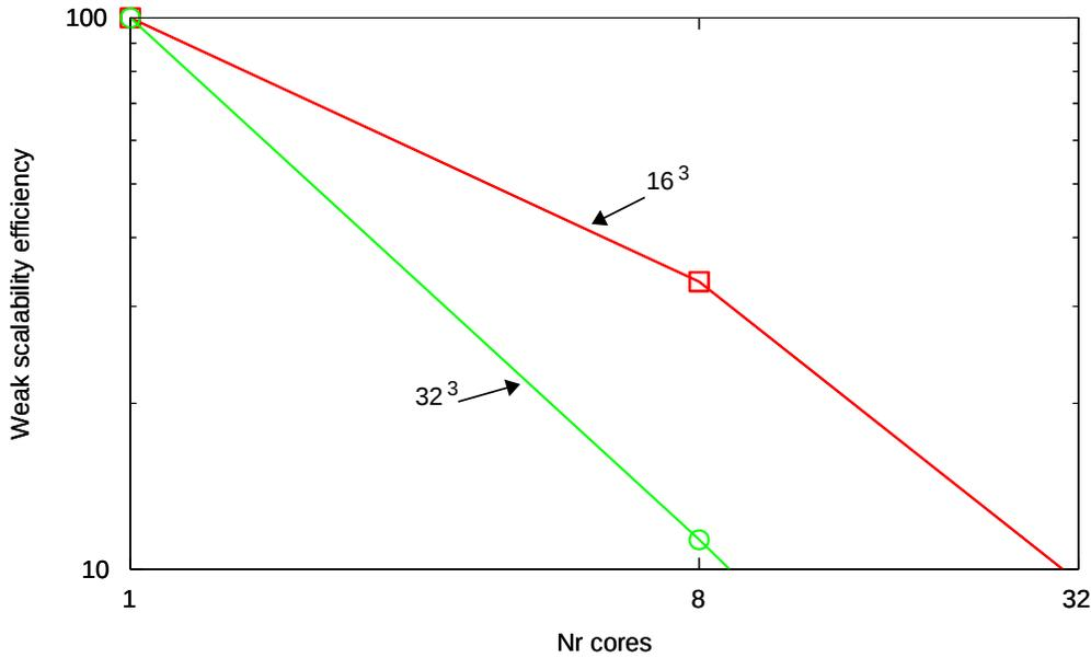
Figure 13: Weak scalability of the MUMPS direct solver for 3D IGA with linear B-splines,  $C^0$  global continuity. Different lines correspond to various problems sizes.
