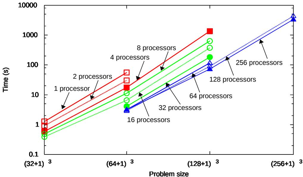
Figure 17: Execution times for the MUMPS direct solver for 3D IGA with linear B-splines,  $C^0$  global continuity.
