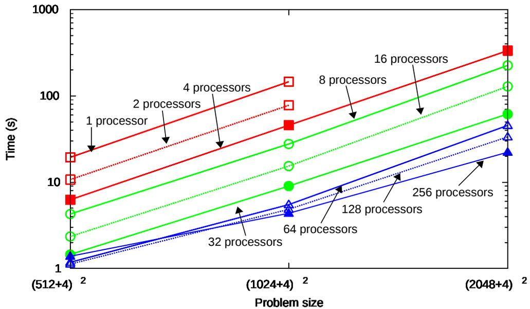
Figure 11: Execution times for the MUMPS direct solver for 2D IGA with quartic B-splines,  $C^3$  global continuity.
