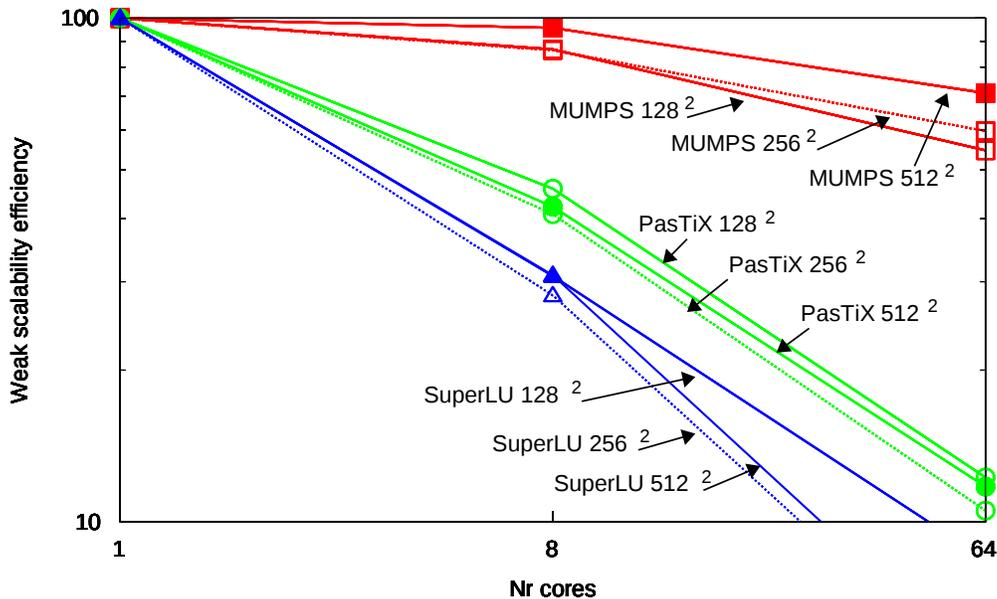
Figure 4: Weak scaling efficiency of the direct solvers for 2D IGA with linear B-splines,  $C^0$  global continuity.
