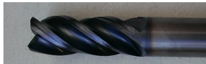
Fig. 1 Tungsten carbide end mills used in the tests
