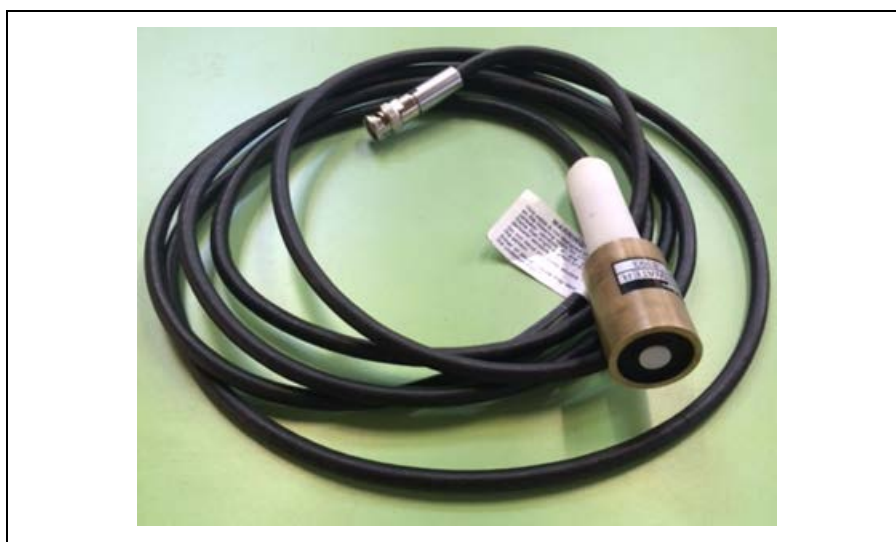
Figure 3-16 Quantum sensor (LI-192SA)
