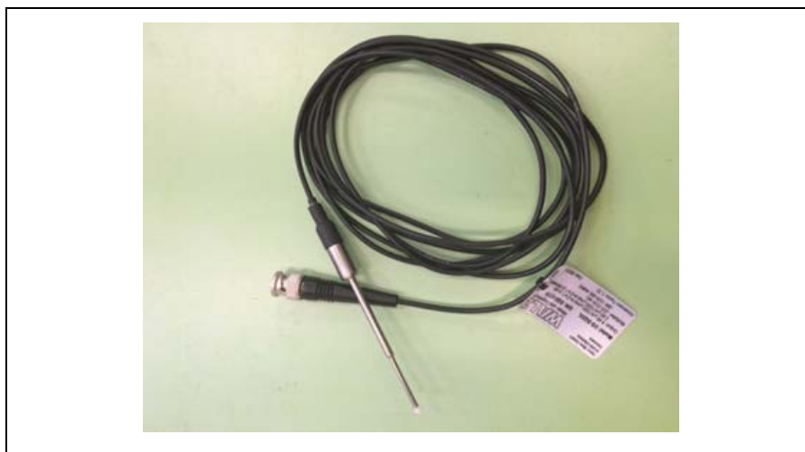
Figure 3-17 Spherical micro quantum sensor (US-SQS/L)
