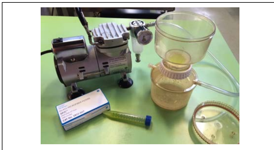
Figure 3-14 Millipore unit and vacuum pump for biomass filtration
