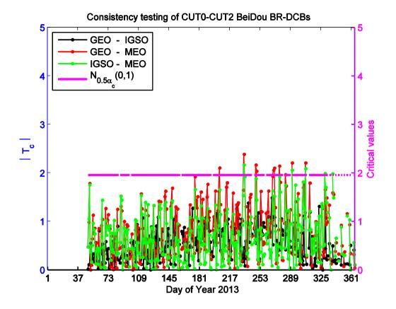
Figure 9. Test statistics  $|T_c|$  (black/red/green dotted lines) used to diagnose the consistency between CUT0-CUT2 GEO/IGSO/MEO BR-DCB estimates (cf. Fig. 8). Critical value  $N_{0.5\alpha_c}$  (0,1) (magenta line) computed using level of significance  $\alpha_c = 5\%$
