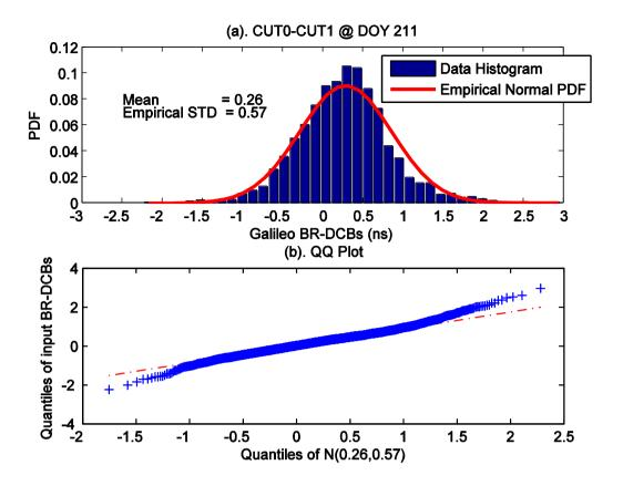
**Figure 4.** *Panel (a)*: The histogram of time-wise Galileo BR-DCB estimates referring to day 211 and receiver-pair of CUT0-CUT1: 2354 samples and 40 bins of width 0.15 ns, and the empirical theoretical normal distribution (*red curve*) based on the mean (0.26 ns) and empirical standard deviation (0.57 ns) of the samples. *Panel (b)*: QQ plot of samples versus normal distribution N(0.26, 0.57)
