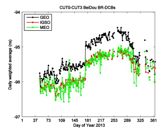
**Figure 6.** The DWA estimates of CUT0-CUT3 (*Trimble-Javad*) BeiDou BR-DCBs in 2013: GEO results (*black dotted line*), IGSO results (*red dotted line*) and MEO results (*green dotted line*)
