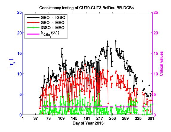
Figure 7. Test statistics  $|T_c|$  (black/red/green dotted lines) used to diagnose the consistency between CUT0-CUT3 GEO/IGSO/MEO BR-DCB estimates (cf. Fig. 6). Critical value  $N_{0.5\alpha_c}$  (0,1) (magenta line) computed using level of significance  $\alpha_c = 5\%$
