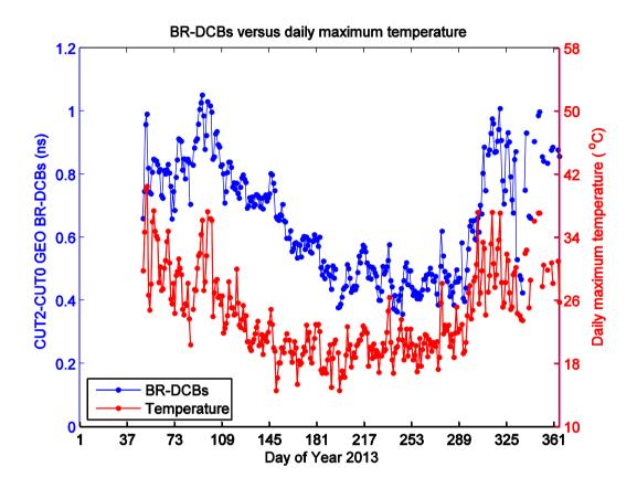
**Figure 11.** The DWA estimates of CUT2-CUT0 GEO BR-DCBs (*blue dotted line*) and the daily maximum temperature values (*red dotted line*) measured by a weather station deployed about 8 km away from the receiver site. The Pearson correlation coefficient between both time series is 0.788 with a corresponding p-value of almost zero
