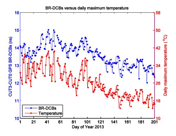
**Figure 12.** The DWA estimates of CUT3-CUT0 GPS BR-DCBs (*blue dotted line*) and the daily maximum temperature values (*red dotted line*) measured by a weather station deployed about 8 km away from the receiver site. The time period indicated by the horizontal axis covers days 1-201 of 2013. The Pearson correlation coefficient between both time series is 0.90 with a corresponding p-value very close to zero
