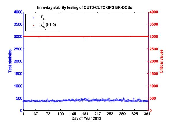
**Figure 3.** Test statistics  $T_s$  (*blue circles*) used to diagnose the intra-day stability in the time-wise estimates of CUT0-CUT2 GPS BR-DCBs. Critical values  $\chi^2_{\alpha_s}(t-1,0)$  (*red dots*) computed using level of significance  $\alpha_s = 5\%$ , together with the degree of freedom (t-1)
