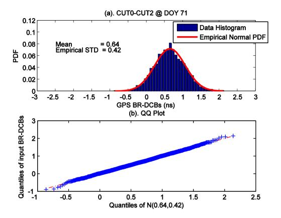
**Figure 5.** *Panel (a)*: The histogram of time-wise GPS BR-DCB estimates referring to day 71 and receiver-pair of CUT0-CUT2: 2880 samples and 40 bins of width 0.15 ns, and the empirical theoretical normal distribution (*red curve*) based on the mean (0.64 ns) and empirical standard deviation (0.42 ns) of the samples. *Panel (b)*: QQ plot of samples versus normal distribution N(0.64, 0.42)
