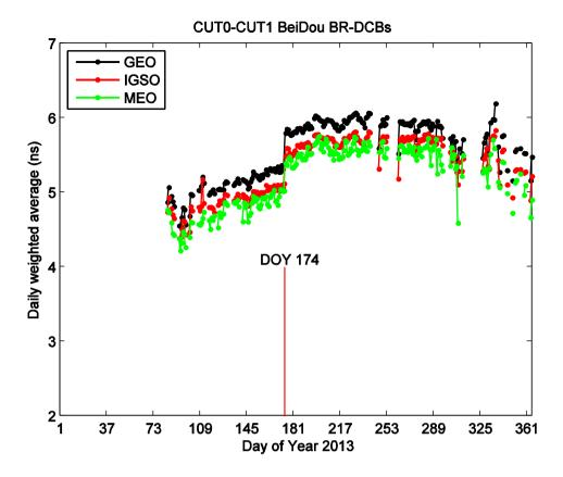
**Figure 10.** The DWA estimates of CUT0-CUT1 (*Trimble-Septentrio*) BeiDou BR-DCBs in 2013: GEO results (*black dotted line*), IGSO results (*red dotted line*) and MEO results (*green dotted line*). Only after day 84, CUT1 starts to receive signals from BeiDou IGSO and MEO satellites. The vertical red line indicates the day (*174*) when the firmware version of CUT0 was upgraded from 4.70 to 4.80
