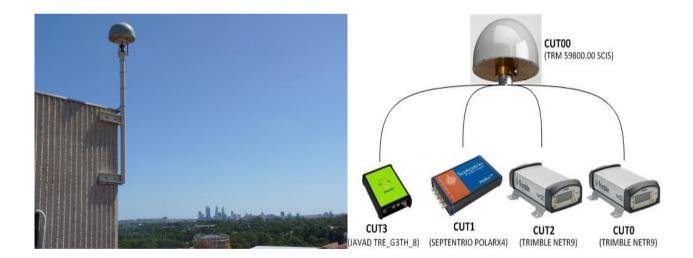
**Figure 1.** Curtin GNSS geodetic grade antenna (*CUT00*) and four multi-GNSS receivers of three types used in this study. *Left*: antenna setup with SCIS radome. *Right*: receiver–antenna connectivity
