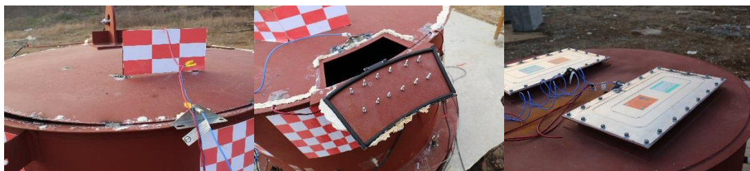
(a) Stitch-Welds for Tank 1 (b) Hinge cover for Tank 2 (c) REMBE vent panel for Tank 3 Fig. 7 Explosion venting installation
