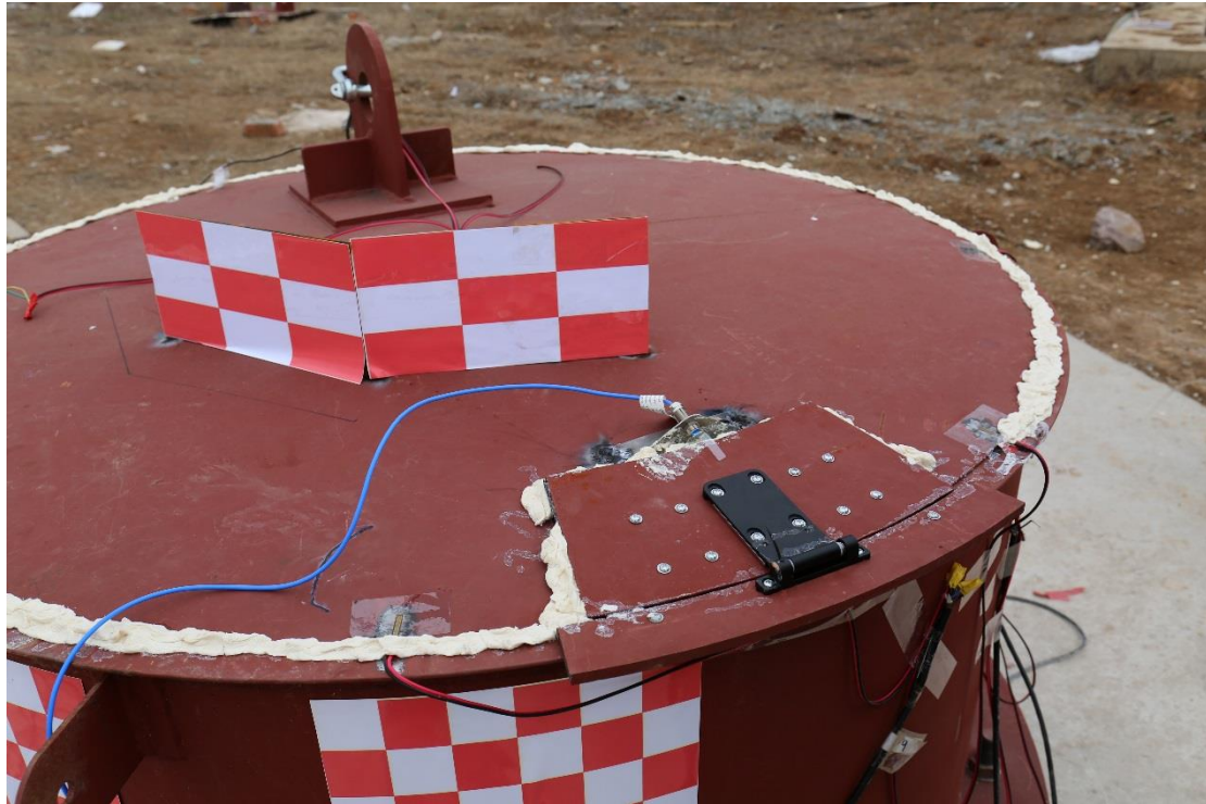
Fig. 3 Latex foam sealant used to seal weld gaps
