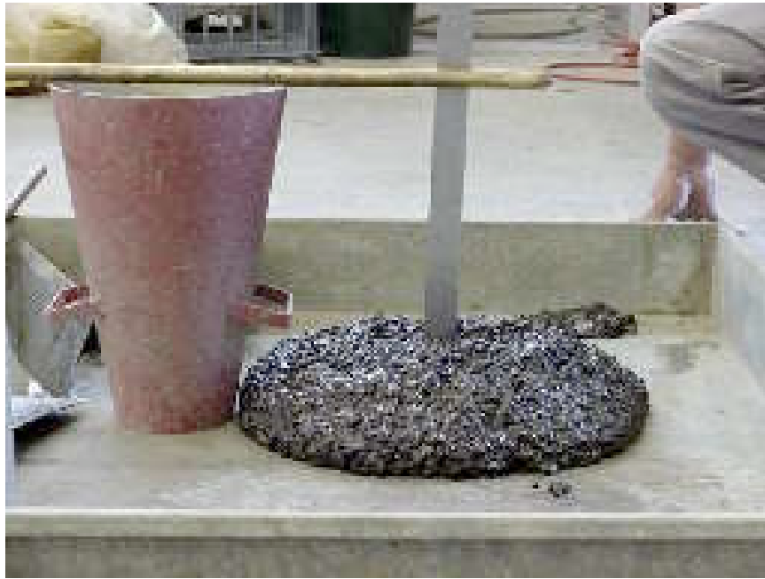
Figure 3.11: Slump Measurement of Fresh Concrete
