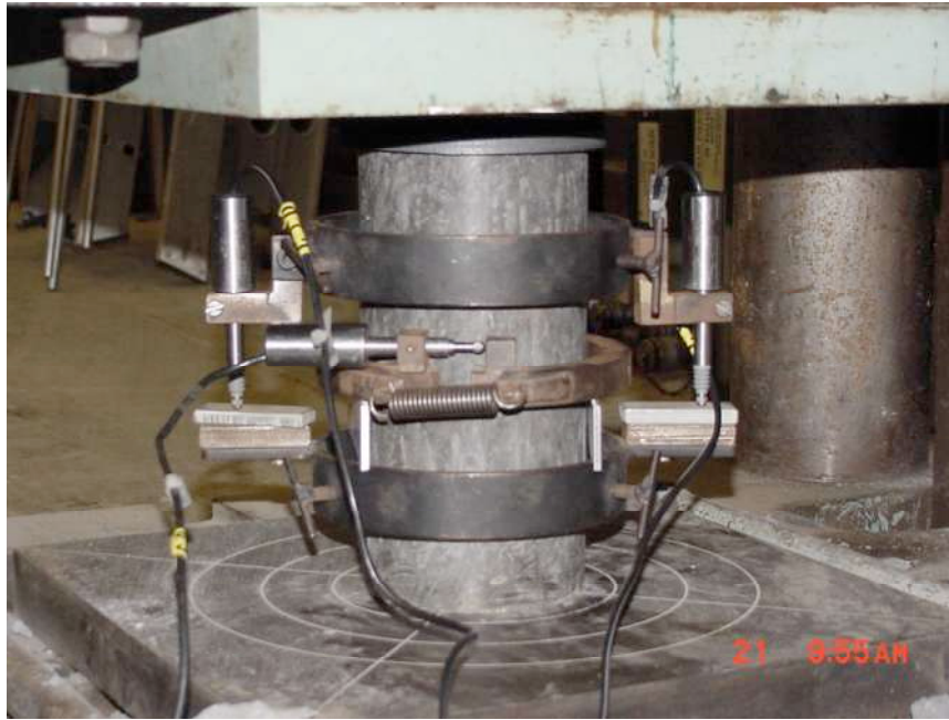
Figure 4.18: Test Set-Up for Measuring the Elastic Constants
