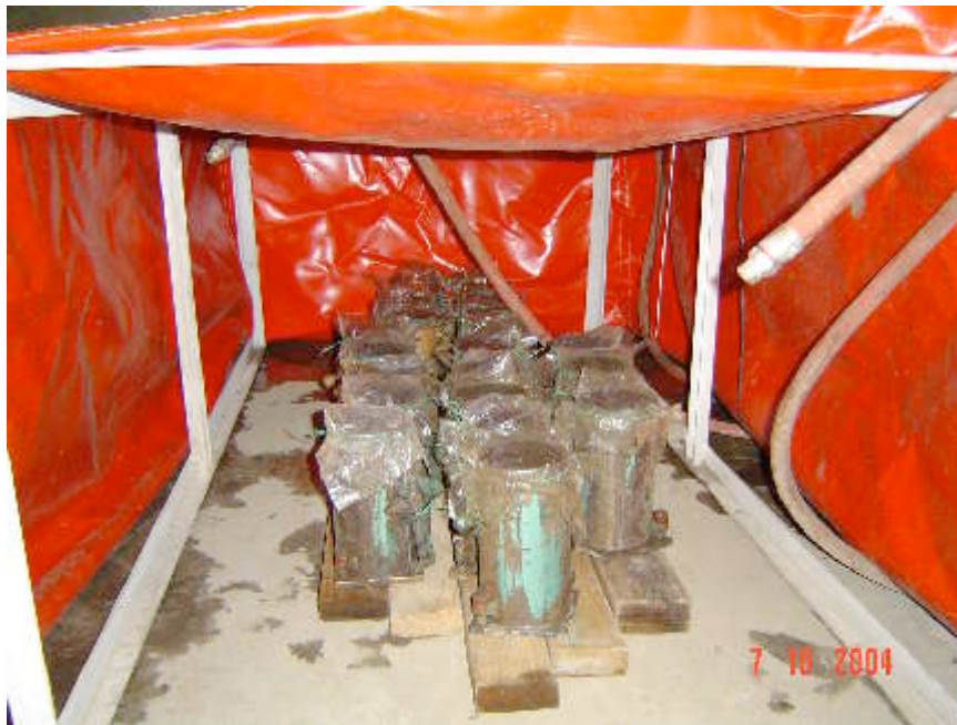
Figure 3.14: Specimens in Steam Curing Chamber
