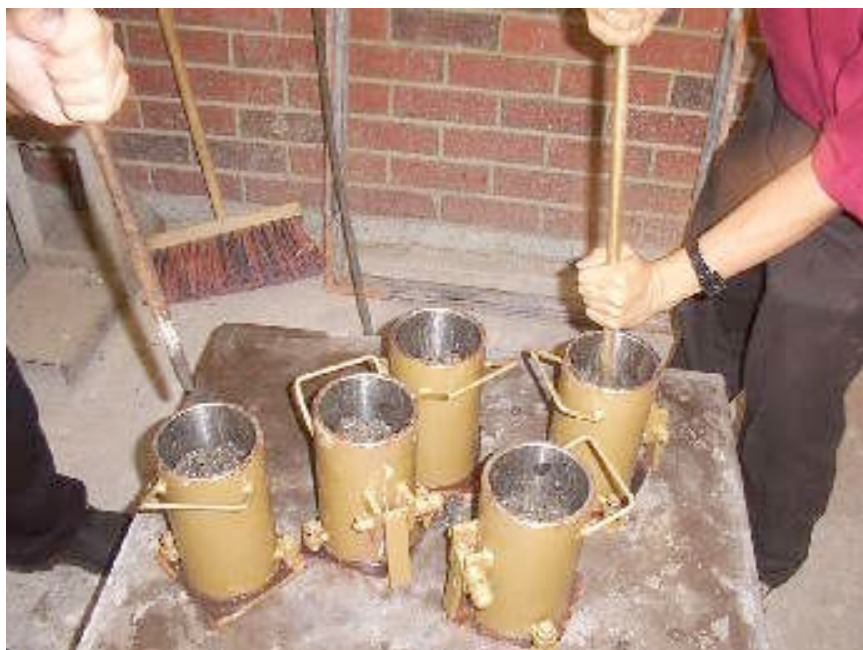
Figure 3.12: Compaction into Moulds
