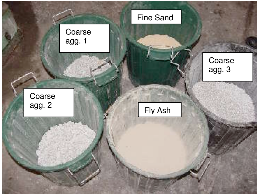
Figure 3.8: Dry Materials for Making Geopolymer Concrete
