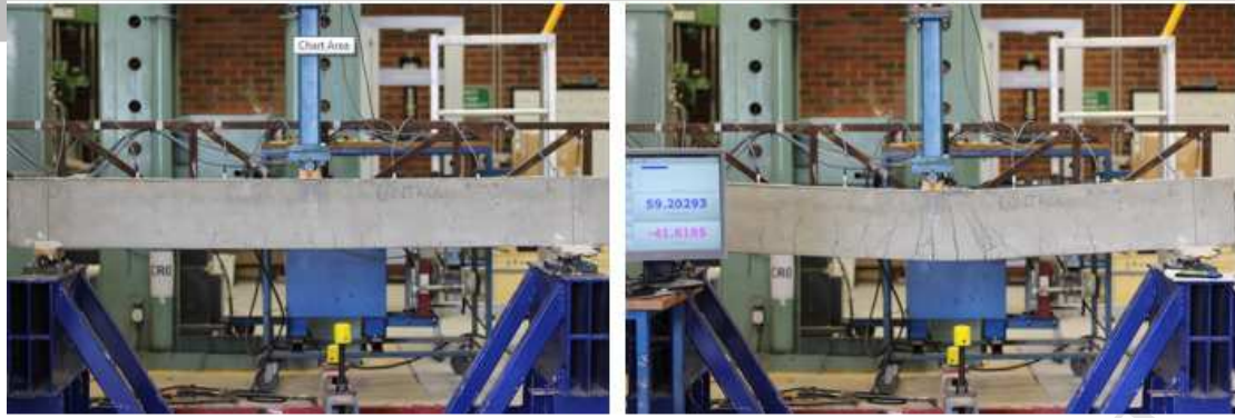
Figure 8 (L) Early crack development of control specimen, (R) Crack development close to failure load of control specimen
