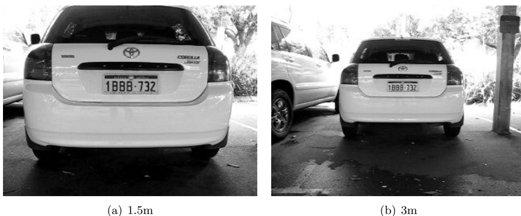
Figure 5.13: Example images of Western Australian number plates. The distance between the camera and the car is about (a) 1.5m and (b) 3m respectively. The resolution of the images is 320 \times 240 pixels.
