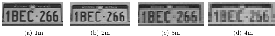
Figure 5.12: Number plate recognition in an indoor environment. The distance between the plate and the camera varies from 1m to 4m. Figures (a) - (d) show cropped images for each distance.
