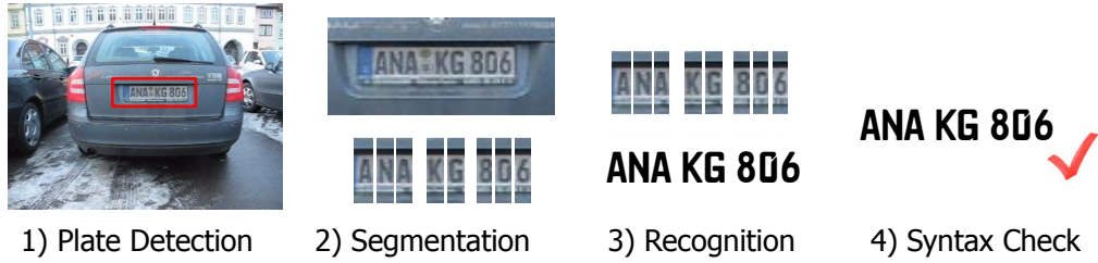
Figure 2.4: The basic steps of number plate recognition methods include plate detection to localise the plate within the image. The cropped plate is then segmented into single characters which are then recognised separately. A syntax check is optional.
