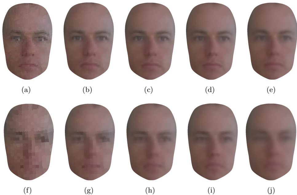
Figure 4.17: Results of the combined tracking and super resolution approach for Person 2 with a face of size 60 \times 40 pixels (top) and 30 \times 20 pixels (bottom) after 1, 20, 50 and 200 frames respectively. The last column ((e) and (j)) shows the result after 200 frames when the input images are interpolated to double the size using bilinear interpolation.
