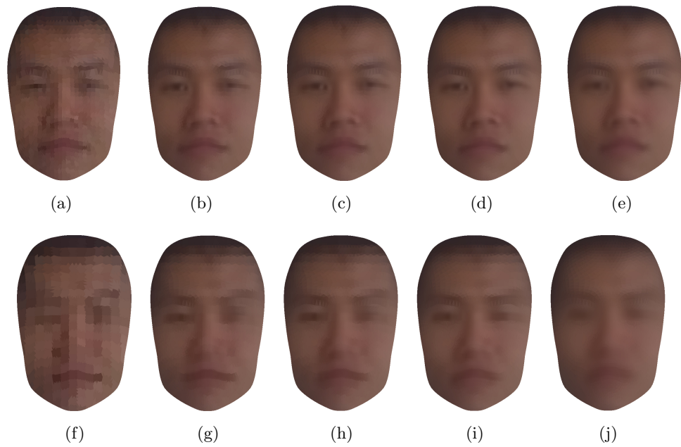
Figure 4.20: Results of the combined tracking and super resolution approach for Person 5 with a face of size 60 \times 40 pixels (top) and 30 \times 20 pixels (bottom) after 1, 20, 50 and 200 frames respectively. The last column ((e) and (j)) shows the result after 200 frames when the input images are interpolated to double the size using bilinear interpolation.
