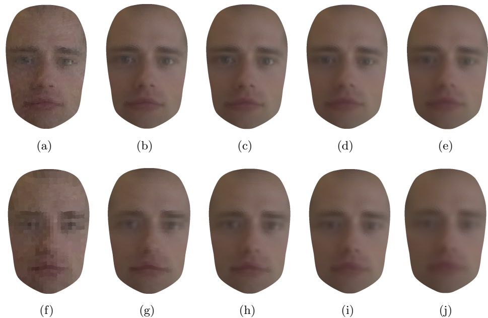
Figure 4.19: Results of the combined tracking and super resolution approach for Person 4 with a face of size 60 \times 40 pixels (top) and 30 \times 20 pixels (bottom) after 1, 20, 50 and 200 frames respectively. The last column ((e) and (j)) shows the result after 200 frames when the input images are interpolated to double the size using bilinear interpolation.
