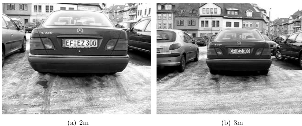
Figure 5.16: Example images of German number plates recorded in an outside car park. The distance between the camera and the car is about (a) 2m and (b) 3m respectively. The resolution is 320 \times 240 pixels.
