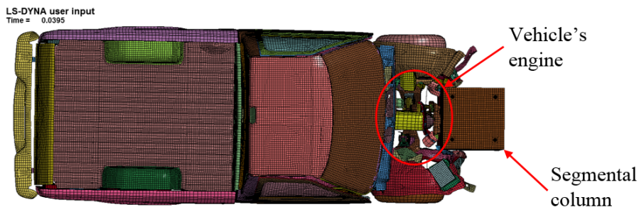
(c) After vehicle's engine hits the column ( t = 39.5 ms)
