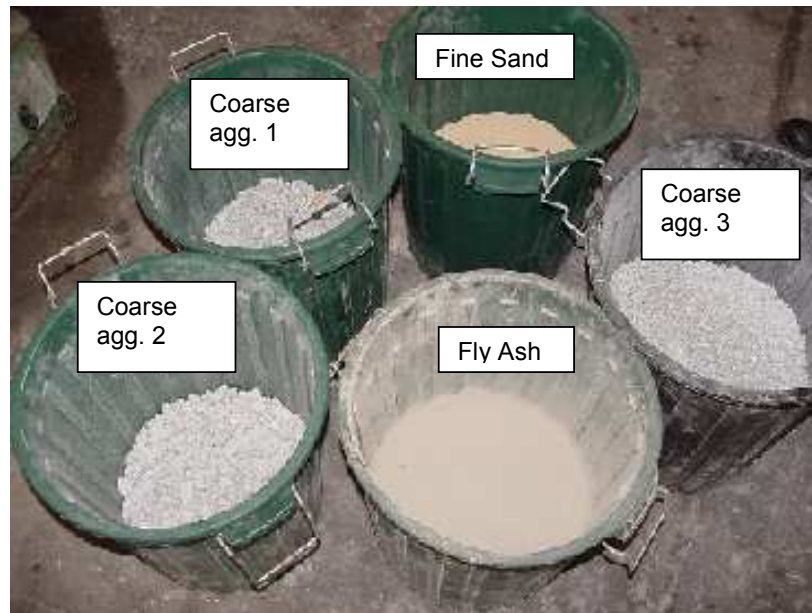
Figure 3.8: Dry Materials for Making Geopolymer Concrete
