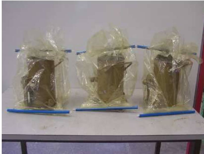
Figure 3.5: Wrapping of Concrete Specimens before Curing (1)
