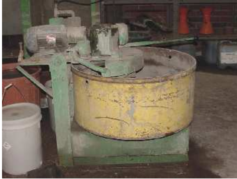
Figure 3.7: Pan Mixer Used for Manufacturing Geopolymer Concrete
