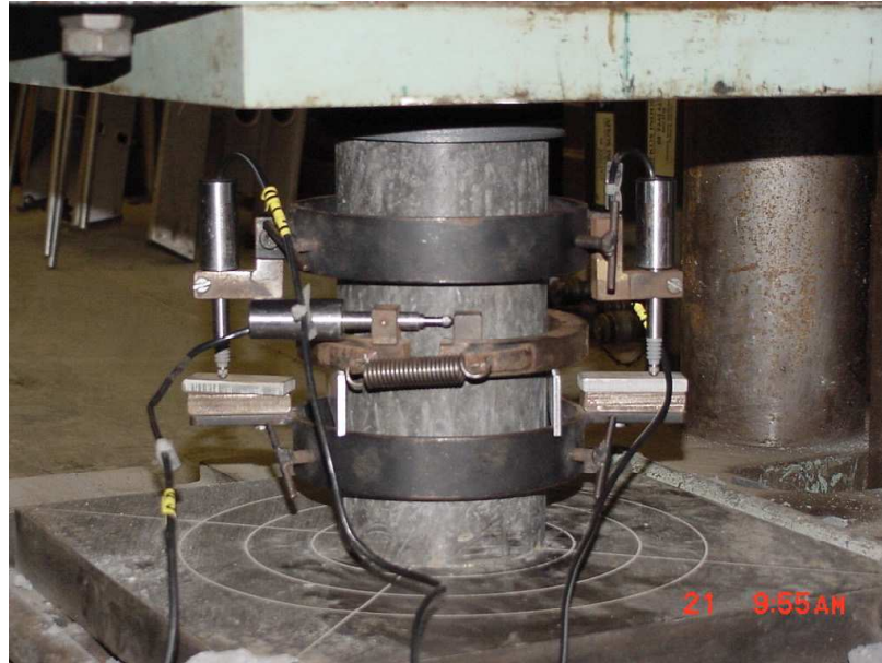
Figure 4.18: Test Set-Up for Measuring the Elastic Constants
