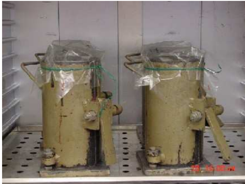
Figure 3.6: Wrapping Concrete Specimens Before Curing (2)
