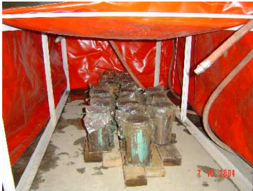
Figure 3.14: Specimens in Steam Curing Chamber
