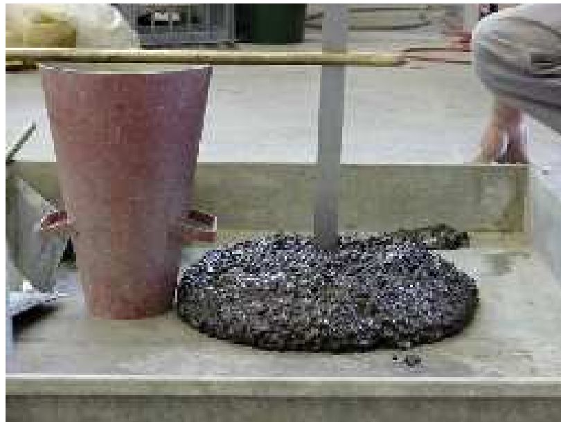
Figure 3.11: Slump Measurement of Fresh Concrete
