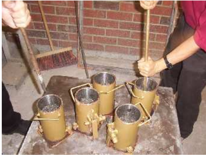
Figure 3.12: Compaction into Moulds
